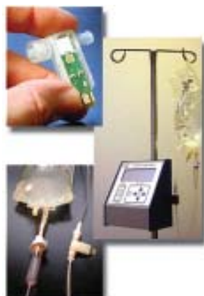
Caption: MEMS flow sensor and single drug prototype sensing unit for IV drug infusions Courtesy of Integrated Sensing Systems, Inc.
