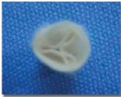
Caption: Elastic biopolymer scaffold for a tissue engineered heart valve
