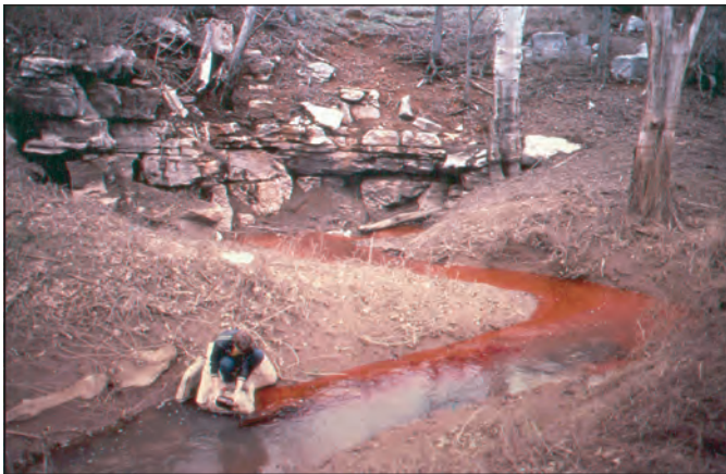
Figure 16. Dye injections: A , sodium fluorescein injection into collapse sinkhole formed in a pond (stream of water is outflow from a settling pond at a public supply water-treatment plant); B , Rhodamine WT injected into sinking stream; C , injection of Rhodamine WT into a water-level observation well (photographs by Charles J. Taylor, U.S. Geological Survey).
