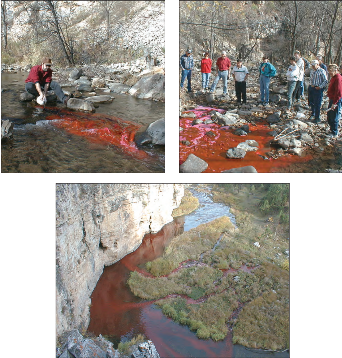
Figure 18. Example of the use of dye to examine water fluxes between surface water and ground water (from Carter and others, 2002). Dye testing has been done in Boxelder Creek, South Dakota, which can lose as much as 50 cubic feet per second of flow to the bedrock aquifers. In the upper left photograph, nontoxic, red dye is poured into Boxelder Creek upstream from a major loss zone. In the upper right photograph, dye in the stream can be seen disappearing into a sinkhole in the Madison Limestone. In the bottom photograph, dye in the stream emerges downstream at Gravel Spring, which is about 671 meters (2,200 feet) (linear distance) from the major loss zone. The length of time for the first arrival of dye to travel this distance is variable depending on flow conditions but generally is about 1 to 2 hours (Strobel and others, 2000). Thus, the ground-water velocity is about 0.3 to 0.6 kilometer per hour (0.2 to 0.4 mile per hour), which is a very fast rate for ground water. Dye also has been recovered at City Springs, which is in the Rapid Creek Basin, about 30 days after injection. This demonstrates that ground-water flow paths are not necessarily restricted by surface-water drainage basins. (Photographs by Derric L. Isles, South Dakota Department of Environment and Natural Resources.)
