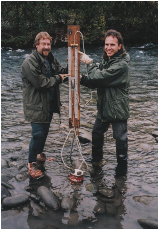
Figure 20. A, Hydraulic potentiometer with users demonstrating hydraulic-head difference between surface water and ground water. The hydraulic head of the river (right side of the board) is higher than the hydraulic head of the ground water (left side of the board), indicating a downward gradient (from Simonds and Sinclair, 2002). Photograph by Kirk A. Sinclair, Washington State Department of Ecology, 2002. B, Components of a hydraulic-potentiometer system (from Winter and others, 1988, copyright 1988 by the American Society of Limnology and Oceanography, Inc., used with permission).
