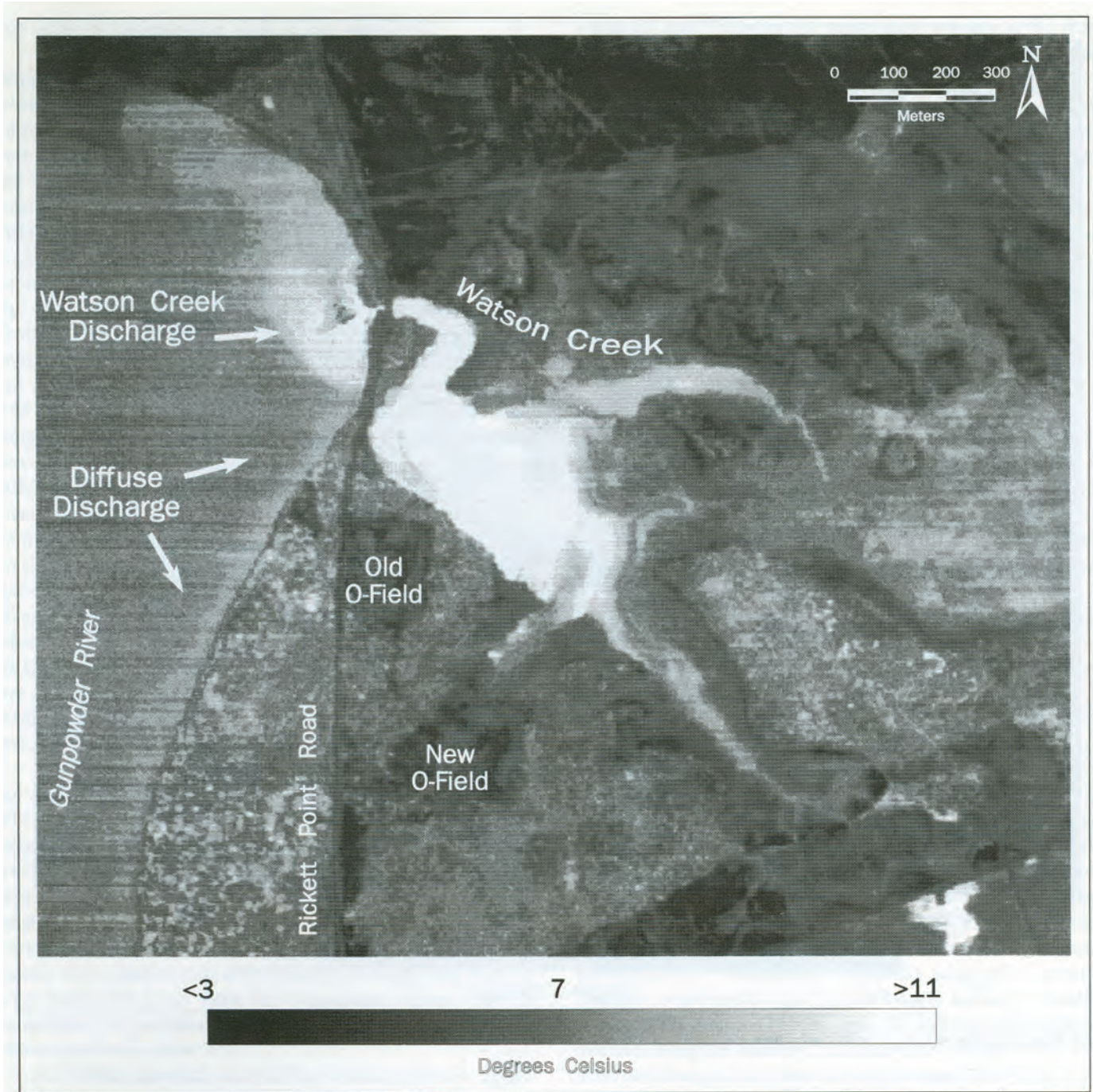
Figure 17. Example of use of thermal infrared imagery to delineate areas of discrete and diffuse ground-water discharge to surface water (from Banks and others, 1996, reprinted from Ground Water with permission from the National Ground Water Association, copyright 1996, thermal imagery of O-Field study area, Aberdeen Proving Ground, Maryland).
