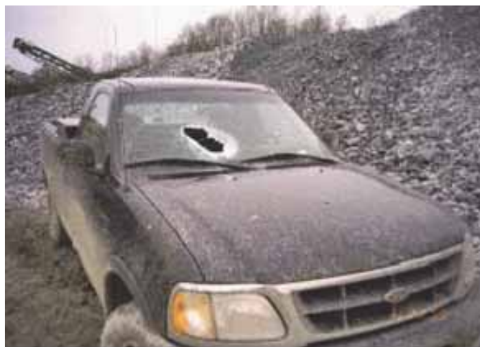
Figure 1.—Example of flyrock damage to a vehicle at a worksite.
