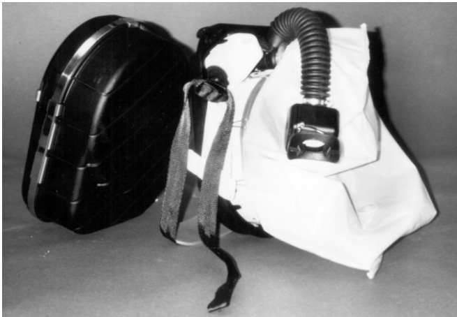
Figure 3.—Cased and uncased Draeger OXY K-Plus self-rescuer.
