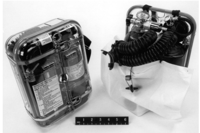
Figure 5.—Cased and uncased Ocenco EBA 6.5 self-rescuer.
