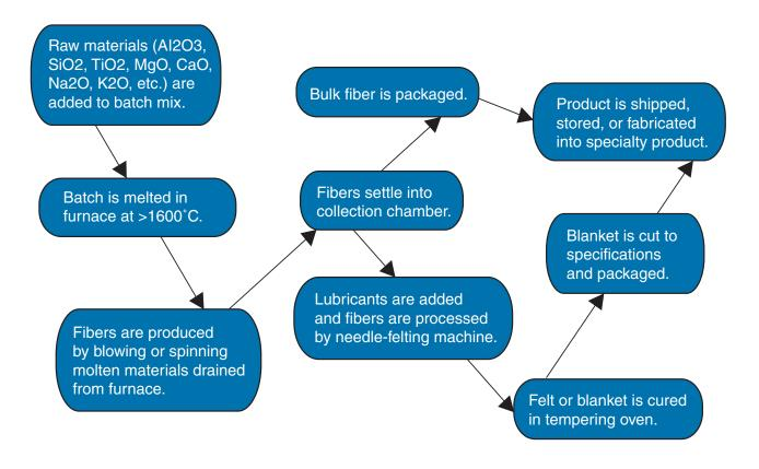
Figure 3–1. Process flow chart for RCF production.
