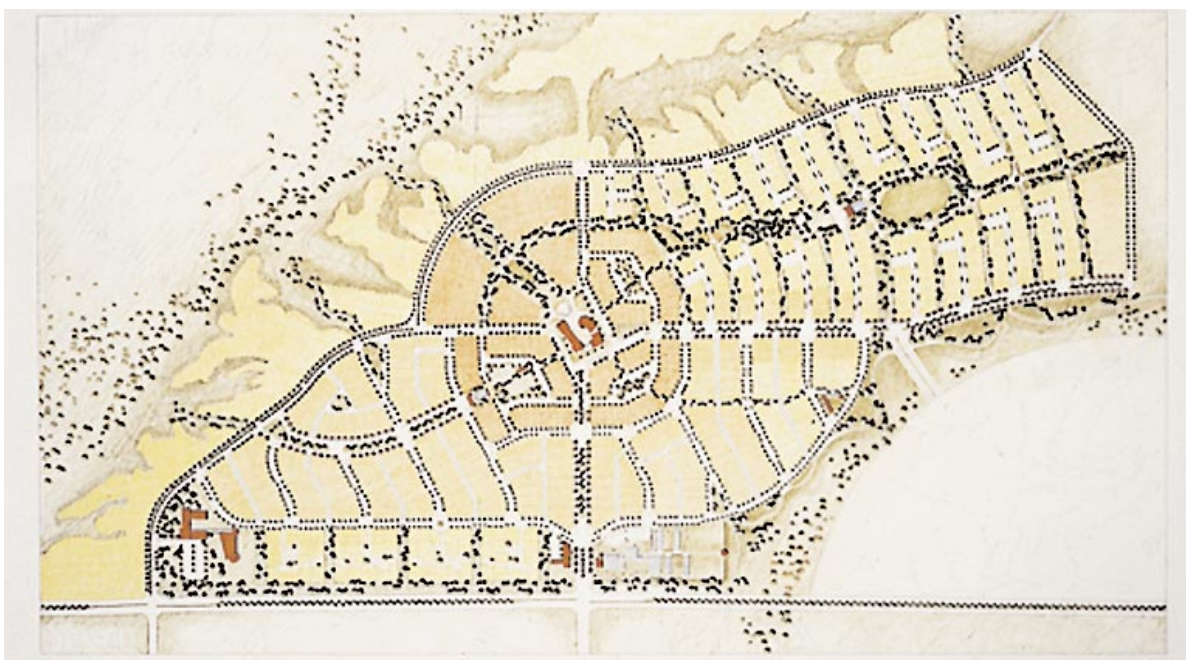
Civano, Arizona. Neighborhood One Plan. The original plan, with its overly rigid road grid system, was modified to respond more sensitively to the landscape and to issues of solar orientation. The neighborhood size evolves from comfortable pedestrian walking distances and the creation of a hierarchy of streets. The streets are designed to ensure that pedestrian traffic would be co-equal with vehicular traffic.
