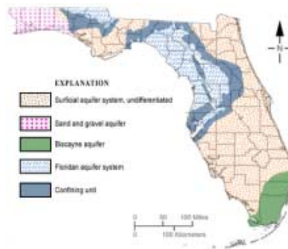
Figure 1. Principal aquifers of Florida exposed at or near the land surface (after Miller 1997).
