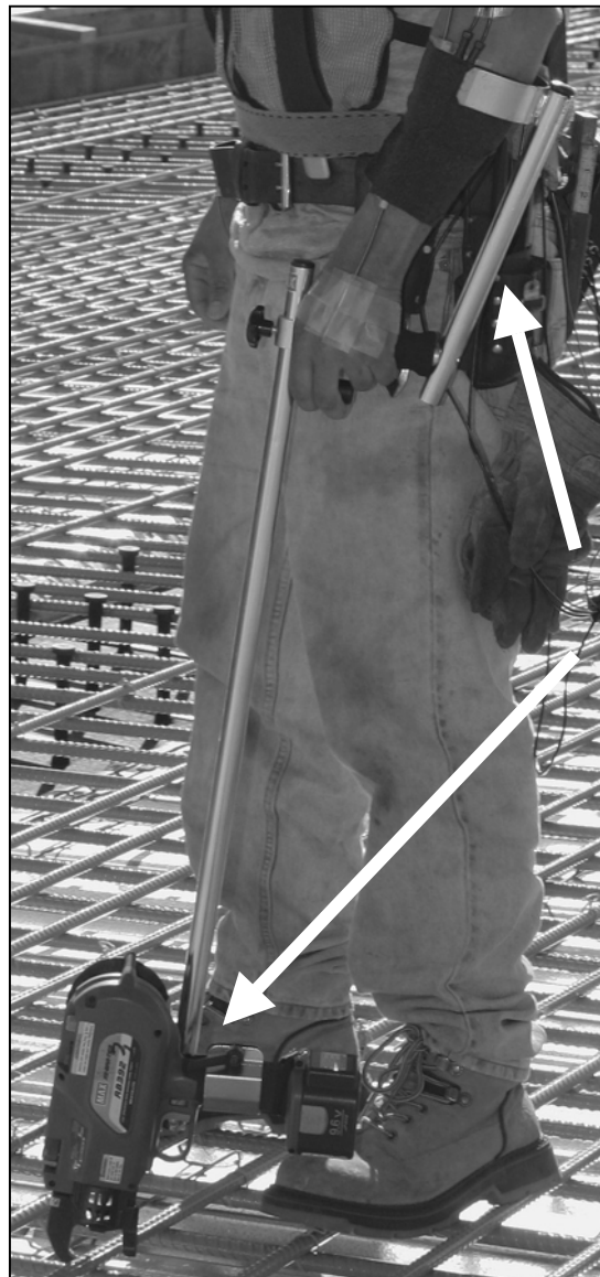
Figure 5 MAX-USA RB-392 Battery powered tier with adjustable extension (BPT+E) (plan to use image from manufacturer)
