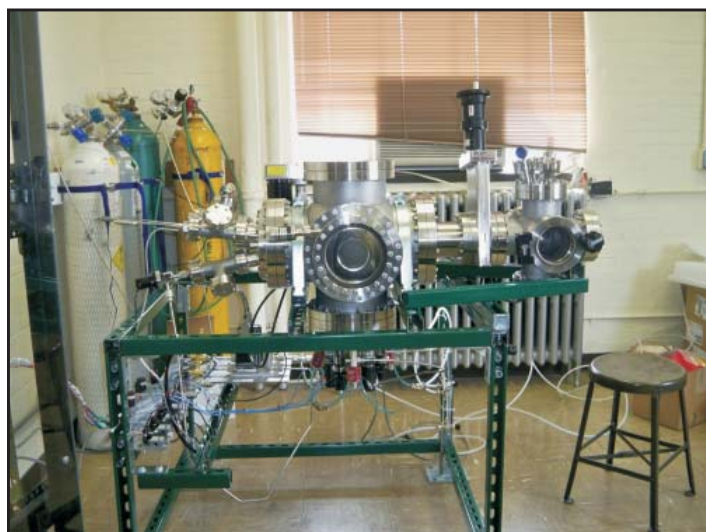
Figure 1. Dedicated thin-film growth facility. The main processing chamber is to the left, load-lock (without transfer mechanism) to the right. The sample stage (not shown) mounts to the top of the main chamber.
