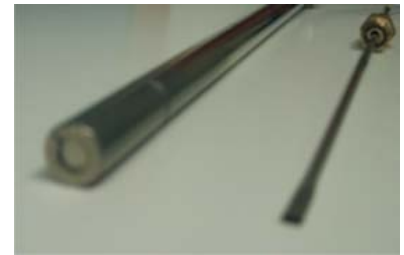
Figure 2. The old 1/2" optical probe (on the left), and the new 1/8" optical probe (on the right).
