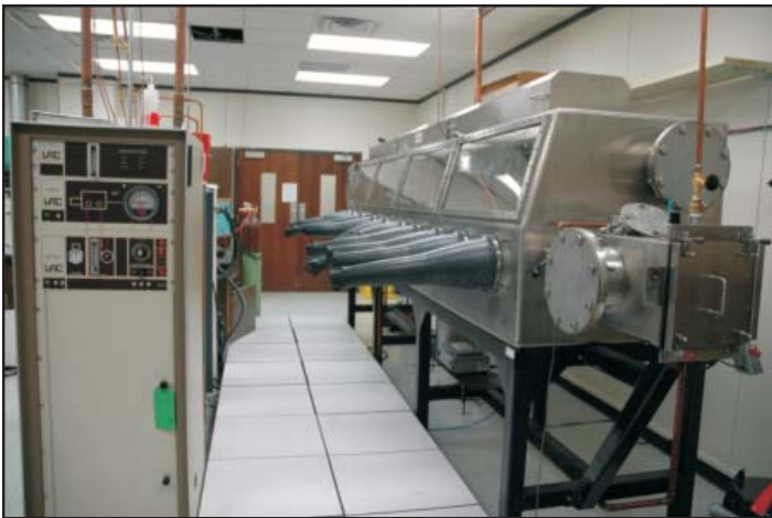
Figure 1. Glovebox installed at Texas A&M University for powder metallurgy of uranium alloys.
