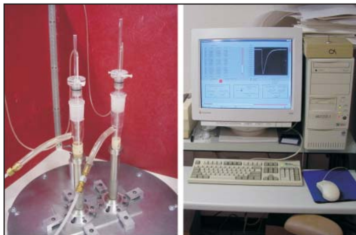
Figure 1. A unique high-temperature calorimeter used for heat measurements of ceramics formation.
