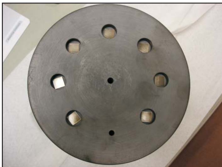
Figure 3. Top view of the silicon carbide block with samples inserted into the seven sample cavities with the black-body cavity at the six o'clock position.
