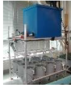
Figure 6. Kreisel larviculture system used to mass culture golden king crab larvae.
