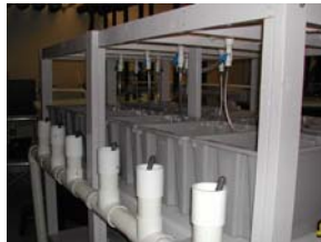
Figure 5. Hatchery system used to collect newly hatched larvae and to estimate hatch timing and daily hatch volumes.
