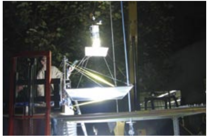
A team demonstrates their concept for a robotic climber that could scale a 200-foot cable powered only by the beam from an industrial searchlight during the 2005 Beam Power Challenge. The challenge was part of NASA's Centennial Challenges. Although none of the 11 teams won the challenge, the University of Saskatchewan Space Design Team had the farthest beam-powered climb, approximately 40 feet. (Photo: NASA/K. Davidian)
