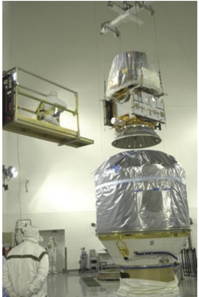
The CALIPSO spacecraft is lowered toward the Lower Delta Payload Attach Fitting at the Astrotech Payload Processing Facility at Vandenberg Air Force Base, California. CALIPSO, a joint project of NASA and the French space agency Centre National d'Etudes Spatiales (CNES), will launch with the Cloudsat satellite in 2006. The satellites will fly in formation as part of the Afternoon Satellite Constellation, or "A-Train," to provide a three-dimensional perspectives of how clouds and aerosols form, evolve, and affect weather and climate. (Photo: NASA)
