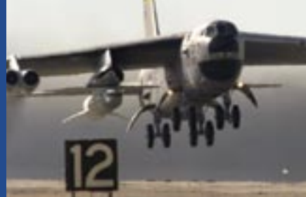
NASA's External Advisors and Partners: NASA's B-52 takes off on November 16, 2004, with a Pegasus booster rocket and the X-43A hypersonic research aircraft tucked under its wing. (Photo: NASA/T. Tschida)
