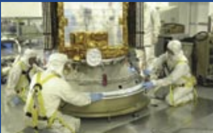
NASA's Strategic Goals: Workers secure the CALIPSO spacecraft onto a payload attach fitting at Vandenberg Air Force Base, California. (Photo: NASA)
