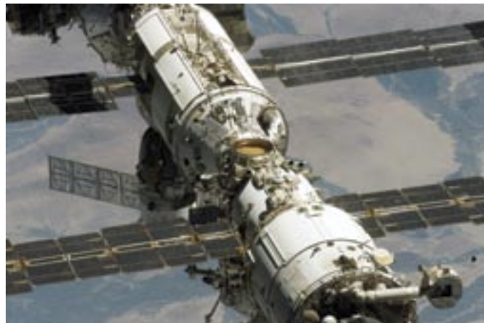
This photograph of the International Space Station was taken during the Shuttle Discovery's fly-around after it undocked on August 5, 2005. Visible are the Zarya module and the Zvezda Service Module. (Photo: NASA)
