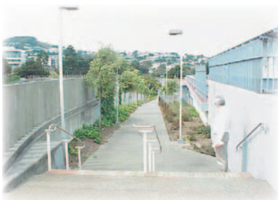
Off-street pedestrian routes, with little or no natural surveillance from windows facing the path, tend to attract few pedestrians, particularly at night. [Balboa Park]
