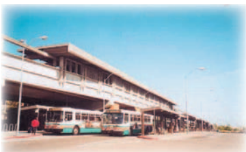
Transfer centers consume valuable land and create “dead” space close to the station, and should therefore be kept as small as possible. Care should be taken not to interpret “ideal” bay requirements and sizes as minimum standards. [El Cerrito del Norte]
