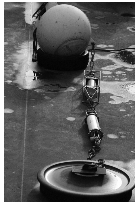
Figure 6. A North Aleutian Basin EAR mooring prior to deployment. Photo by Desray Reeb.
