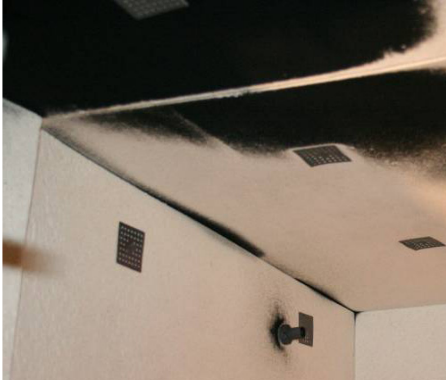
Figure 68. Photo of rear gas sample location after test #6.5 with natural gas using Kaowool M-Board.
