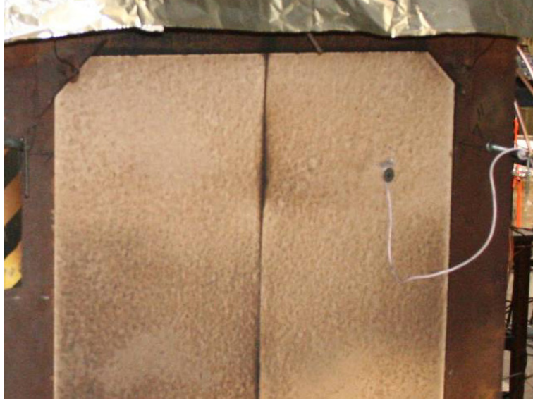
Figure 14. Type K thermocouple attached to the outer surface of the compartment.
