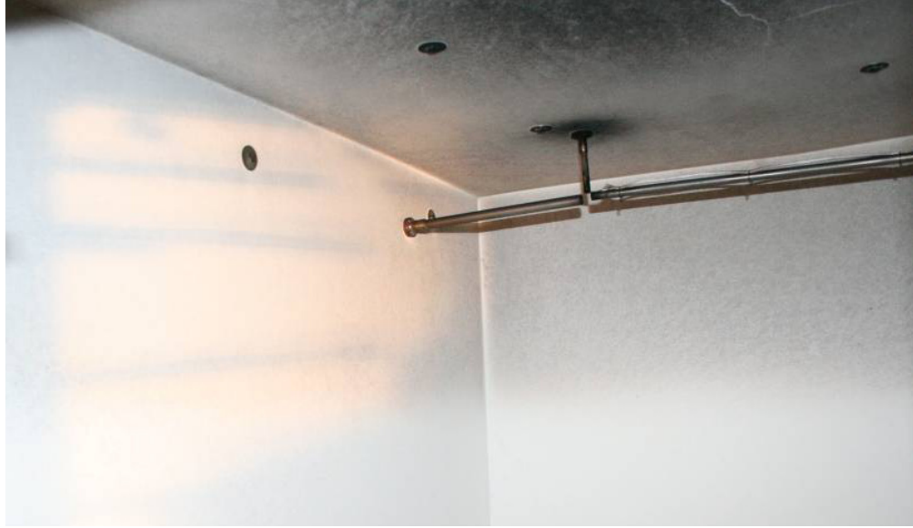
Figure 64. Photo of rear gas sample location and Marinite I construction before test #2.
