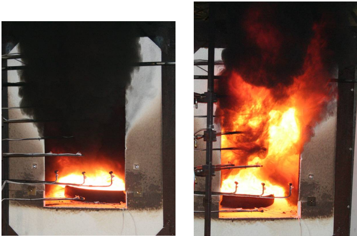
Figure 22. Photographs of polystyrene test #16: t = 389 s, HRR = 170 kW (left), t = 515 s, HRR = 340 kW (right).
