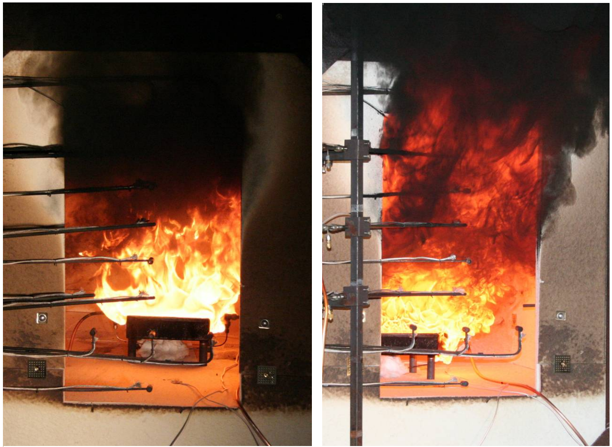
Figure 24. Photographs of toluene pool fire (test #10): t = 1279 s, HRR = 60 kW (left), t = 3843 s, HRR = 200 kW (right).
