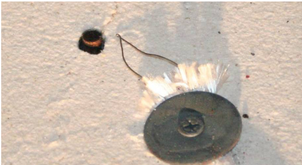
Figure 13. Type K thermocouple on compartment floor surface near a 6 mm diameter total heat flux gauge.
