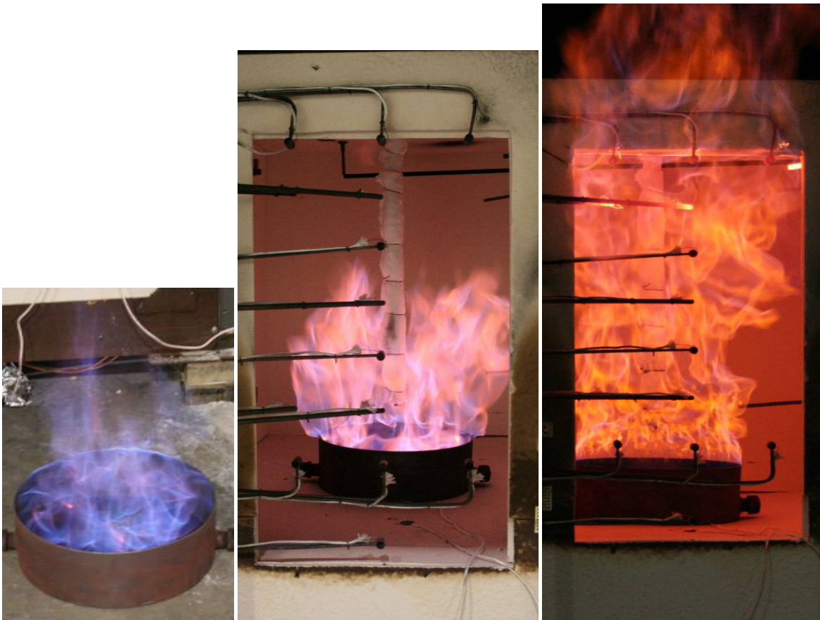
Figure 20. Photographs of methanol test #12: Open burn, HRR = 50 kW (left), t = 645 s, HRR = 72 kW (middle), t = 2885 s, HRR = 305 kW (right).
