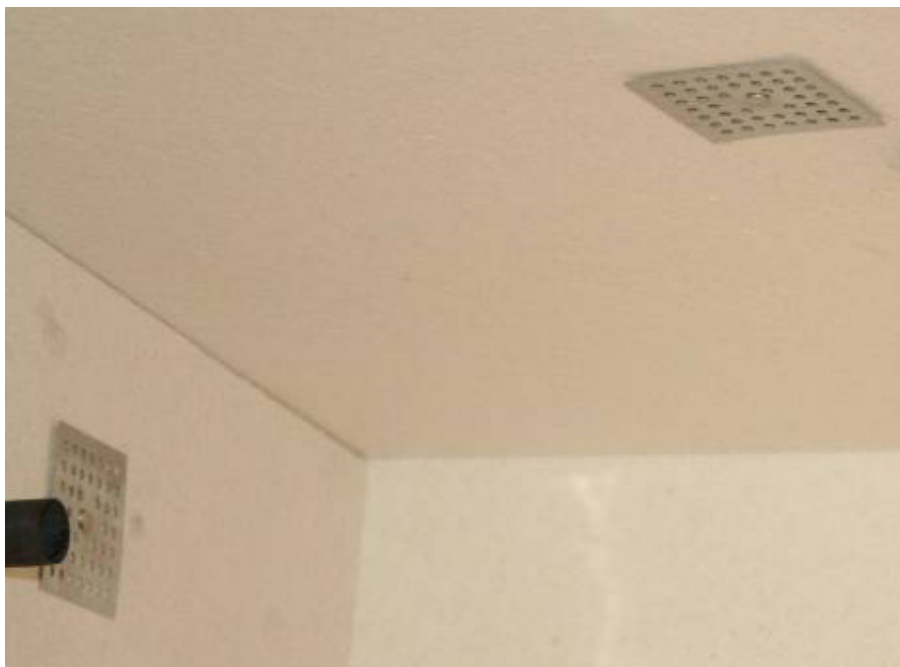
Figure 67. Photo of rear gas sample location showing Kaowool M-board and furnace pin construction prior to test #6.5.
