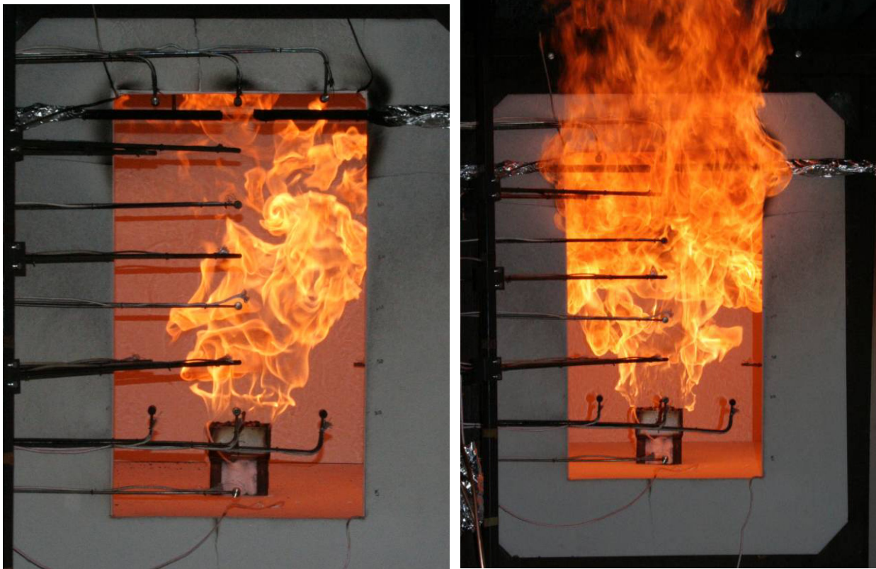
Figure 18. Photograph of test #3 natural gas, HRR = 75 kW (left), HRR = 400 kW (right).
