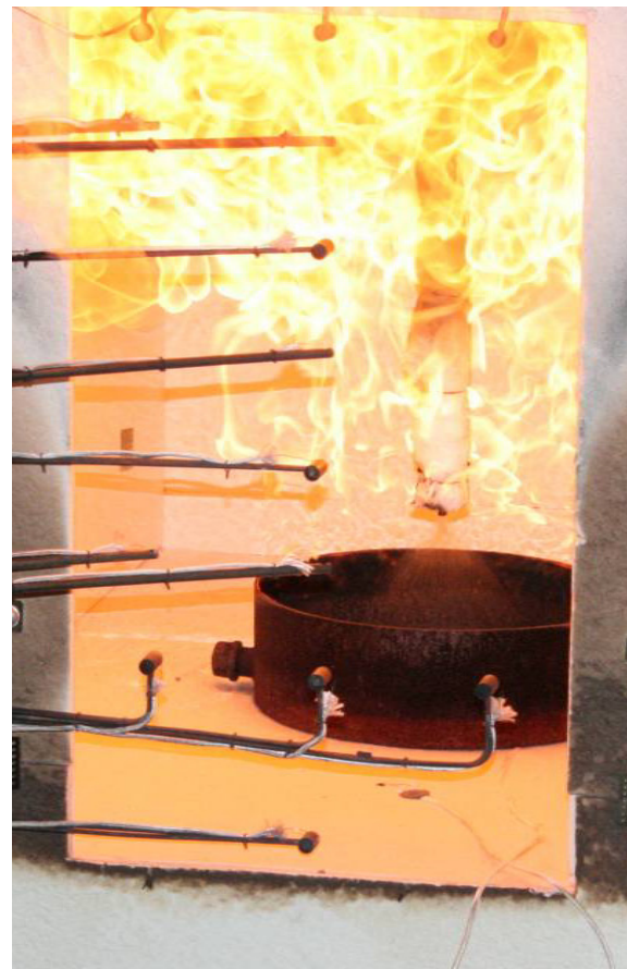
Figure 26. Photographs of ethanol test #11: t = 1709 s, HRR = 145 kW (left), t = 3328 s, HRR = 328 kW (right).
