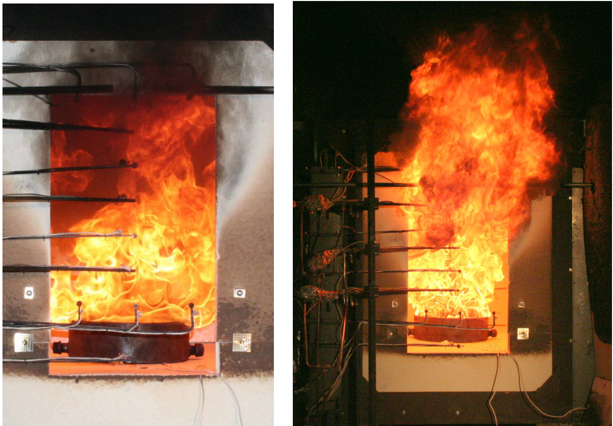
Figure 28. Photographs of heptane test #15: t = 1000 s, HRR = 160 kW (left), t = 2870 s, HRR = 370 kW (right).
