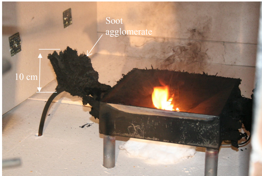
Figure 62. Photograph of soot agglomerate on the water inlet tube of the burner after toluene pool fire (test #10).
