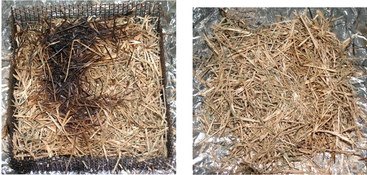
Figure 50. Bottom (left) and top (right) views of an August tall fescue fuel bed are shown after the fuel was removed from the heated plate held at 320 °C with a high wind applied. No glowing combustion was observed.
