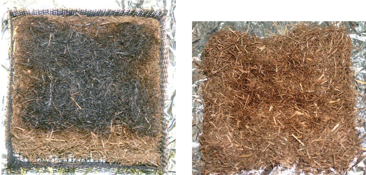
Figure 58. Bottom (left) and top (right) views of a fine Florida grass fuel bed are shown after the fuel was removed from the heated plate held at 310 °C with no wind applied. Glowing combustion was not observed.
