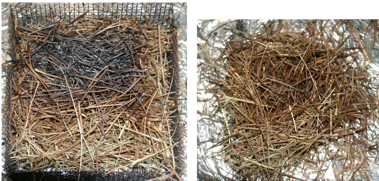
Figure 67. Bottom (left) and top (right) views of a May tall fescue/pine needle mixed fuel bed are shown after the fuel was removed from the heated plate held at 280 °C with no wind applied. No glowing combustion was observed.
