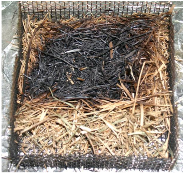
Figure 47. Bottom (left) and top (right) views of an August tall fescue fuel bed are shown after the fuel was removed from the heated plate held at 300 °C with no wind applied. No glowing combustion was observed.
