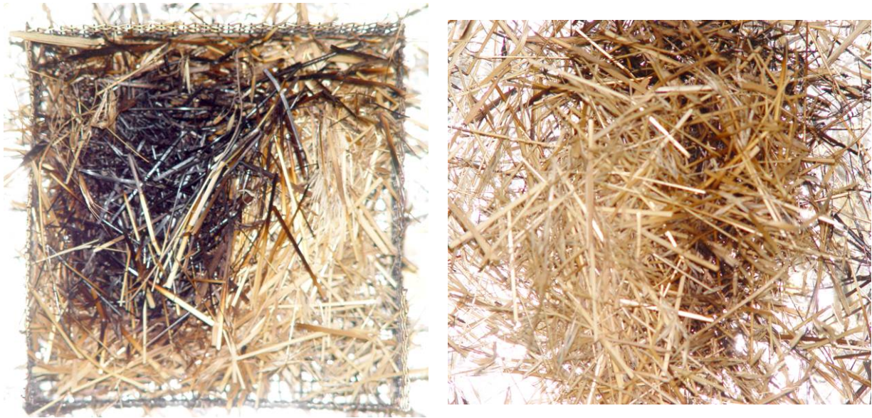
Figure 53. Bottom (left) and top (right) views of a cheat grass fuel bed are shown after the fuel was removed from the heated plate held at 350 °C with a low wind applied. No glowing combustion was observed.
