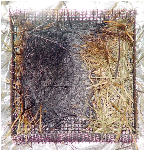
Figure 35. Bottom (left) and top (right) views of a May tall fescue fuel bed are shown after the fuel was removed from the heated plate held at 336 °C with a high wind applied. Glowing combustion was observed after 134 s.
