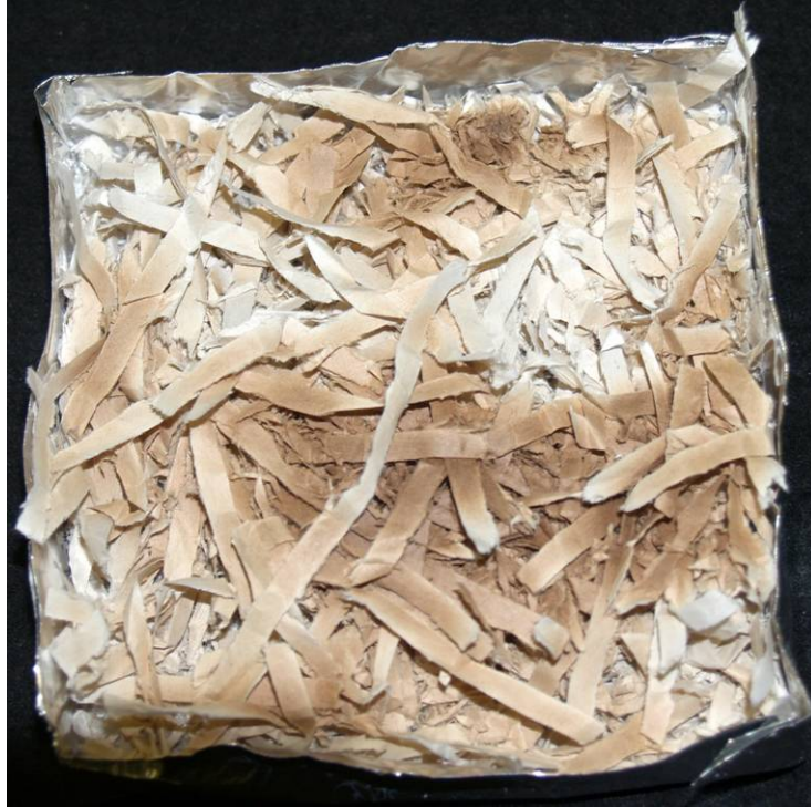
Figure 32. Photograph of the top surface of a shredded newsprint fuel bed following application of a 7.5 \text{ kW/m}^2 heat flux.
