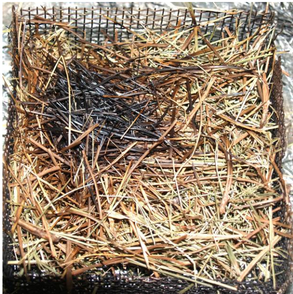
Figure 68. Bottom (left) and top (right) views of a May tall fescue/pine needle mixed fuel bed are shown after the fuel was removed from the heated plate held at 320 °C with a high wind applied. No glowing combustion was observed.
