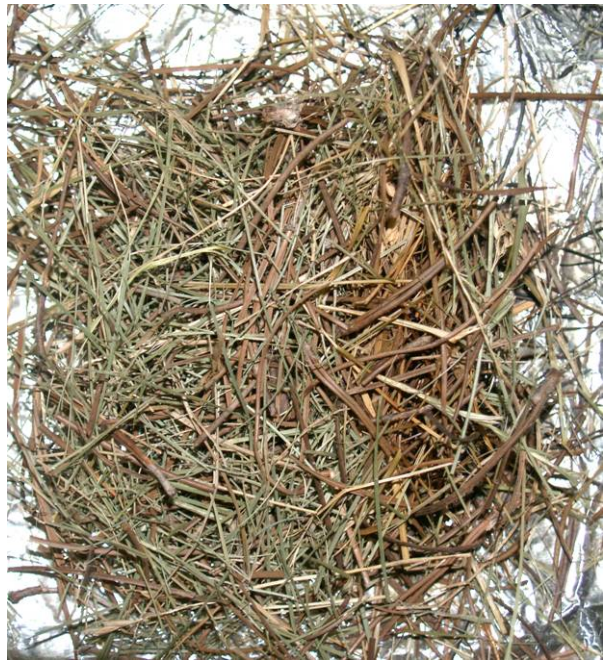
Figure 68. Bottom (left) and top (right) views of a May tall fescue/pine needle mixed fuel bed are shown after the fuel was removed from the heated plate held at 320 °C with a high wind applied. No glowing combustion was observed.
