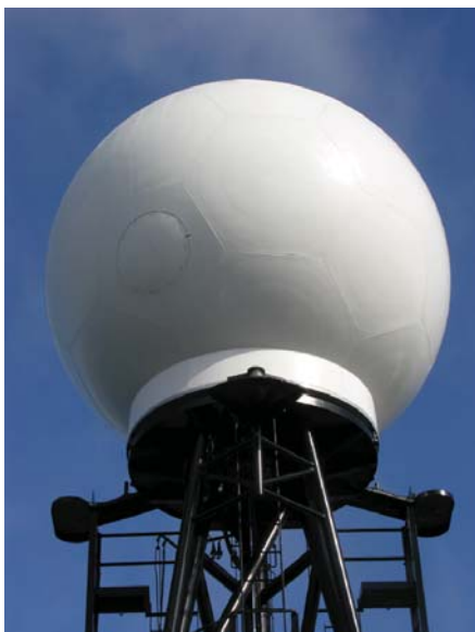
The Very High Speed Aperture Terminal satellite dome will be used to transmit data to shore
