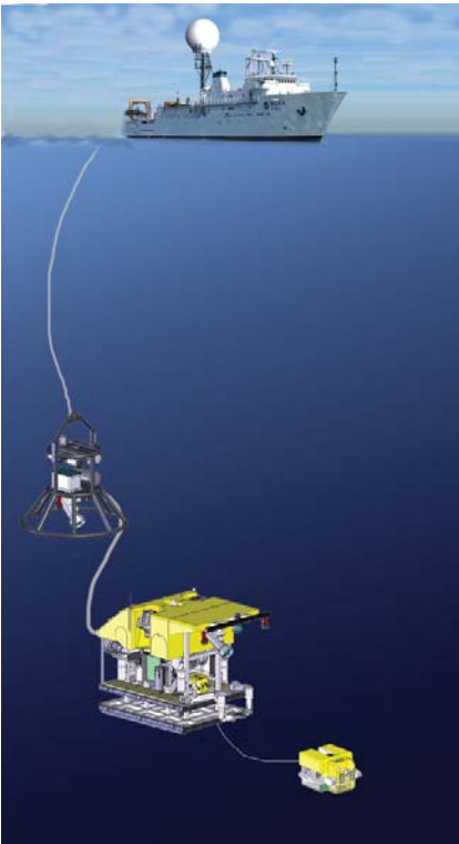
The camera and ROV will transmit data to the ship in real time.
