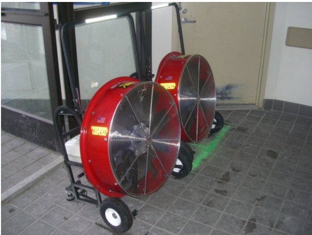
Figure 1.7-1. Front View of PPV Fans
