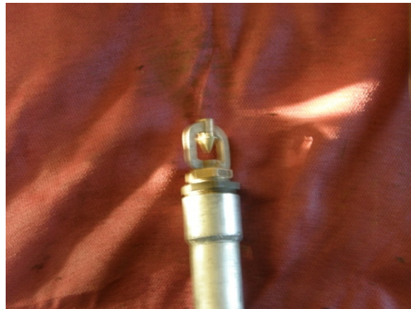
Figure 1.9-4. FBN 2 with a Fog Nozzle (Sprinkler)
