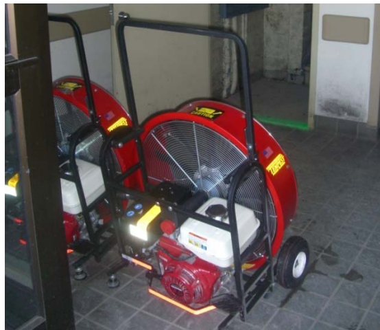
Figure 1.7-2. Rear View of PPV Fans
