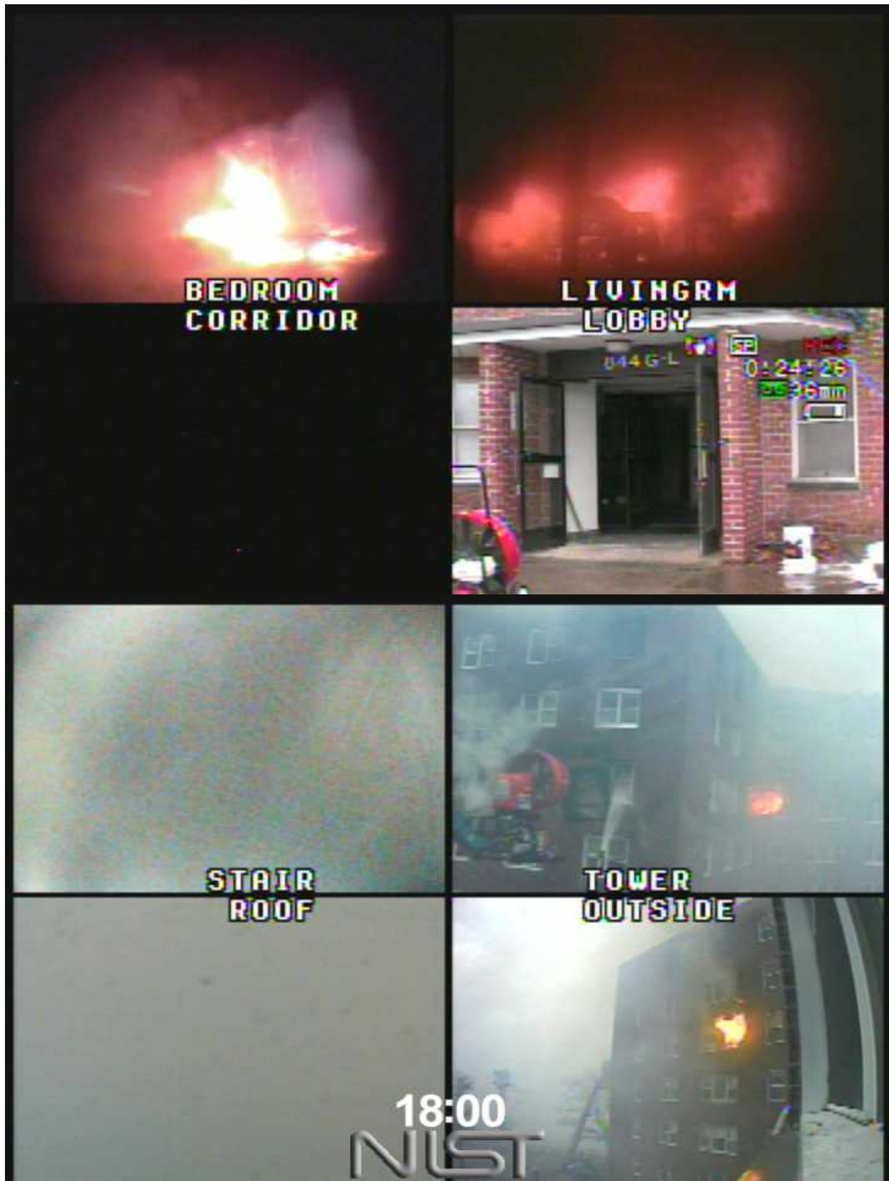
Figure 3.8-11. Experiment 5K, 1080s after ignition.
