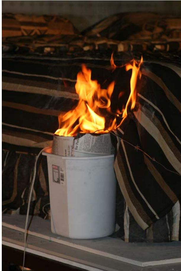
Figure 3.3-4. Trash container ignition of bed fuel package.
