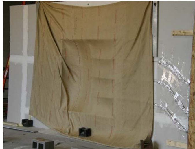
Figure 4.3.2-2. Large WCD deployed over window opening.
