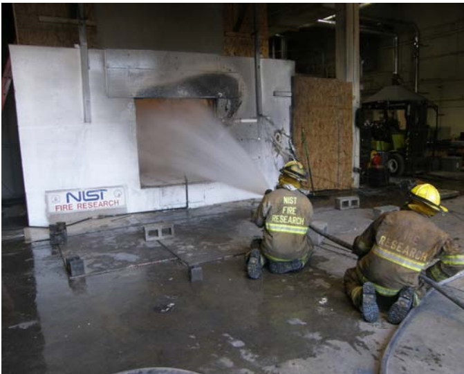
Figure 4.3.3-3. Fog stream discharged into window opening.
