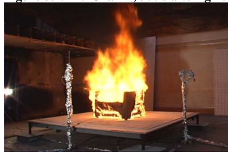
Figure 3.4.1-6. Chair 1, at peak heat release rate, 417 s after ignition
