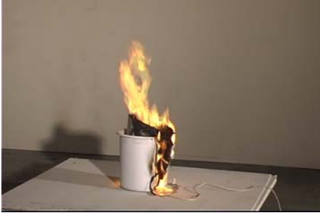
Figure 3.2-11. Trash container 2, 200 s after ignition
