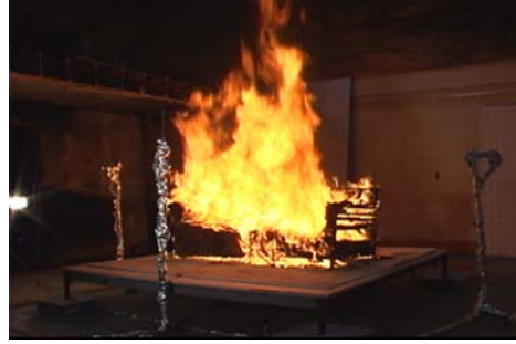
Figure 3.5-6. Sofa 1, at peak heat release rate, 455 s after ignition
