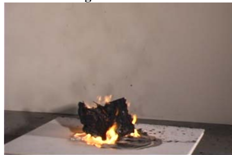
Figure 3.2-8. Trash container 1, 600 s after ignition
