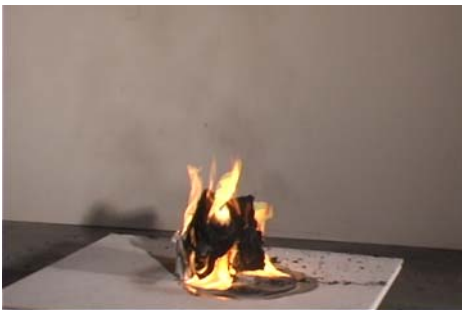
Figure 3.2-7. Trash container 1, 500 s after ignition
