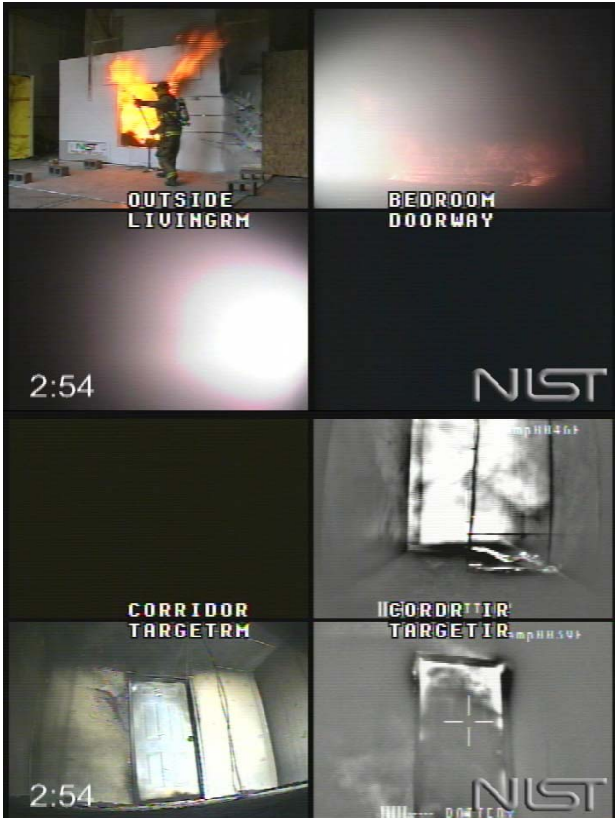
Figure 5.6.1-4. Experiment 6, window fully vented, 174 s after ignition.
