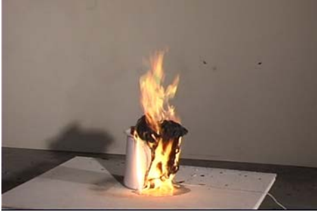
Figure 3.2-3. Trash container 1, 200 s after ignition
