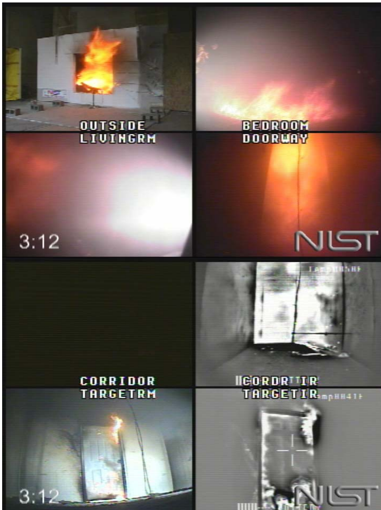
Figure 5.6.1-6. Experiment 6, corridor flames, 192 s after ignition.
