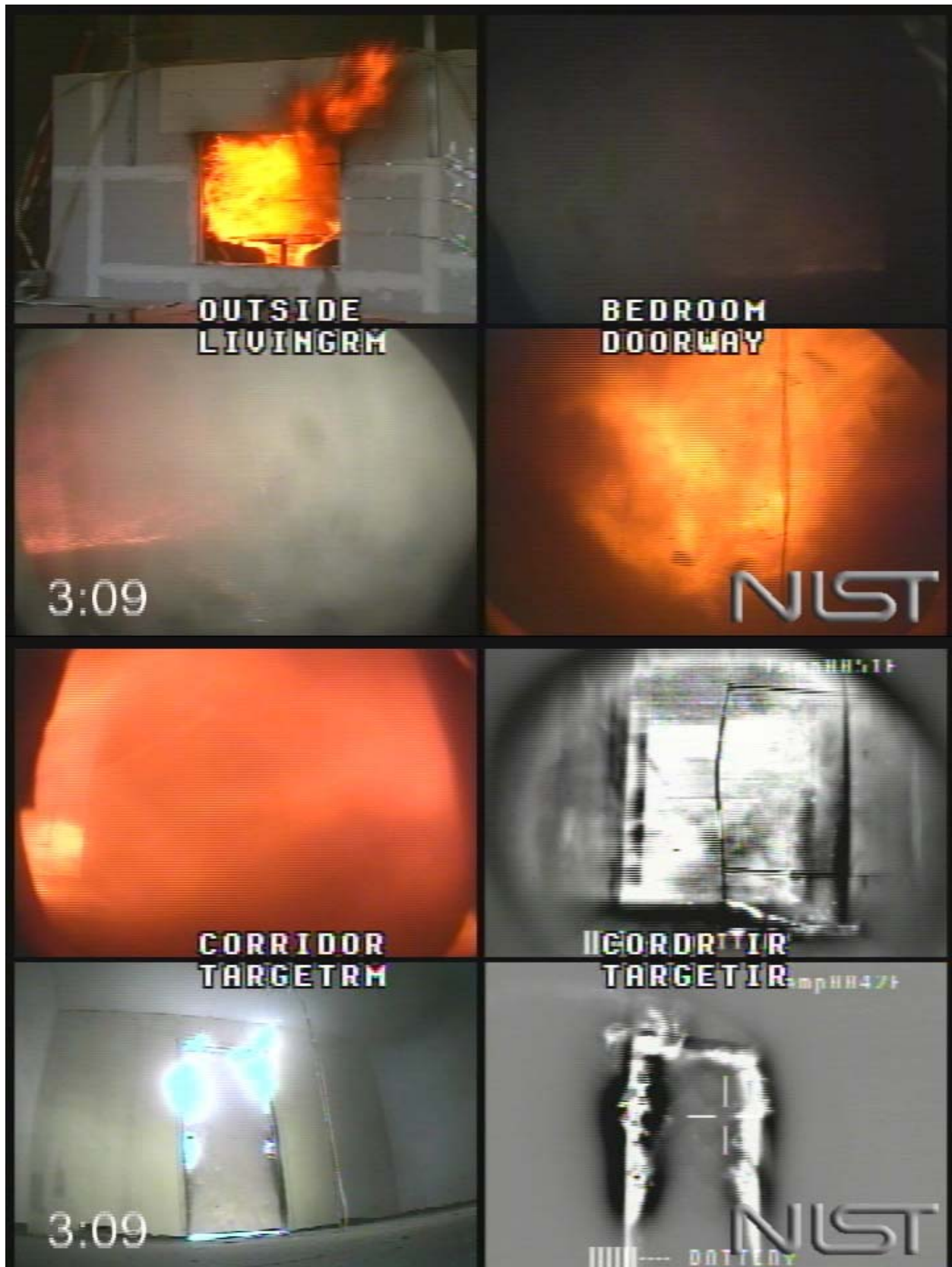
Figure 5.2.1-5. Experiment 2, corridor flames, 189 s after ignition.
