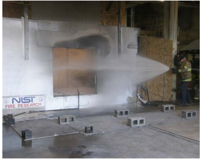
Figure 4.3.3-2. Fog stream discharged across window opening.
