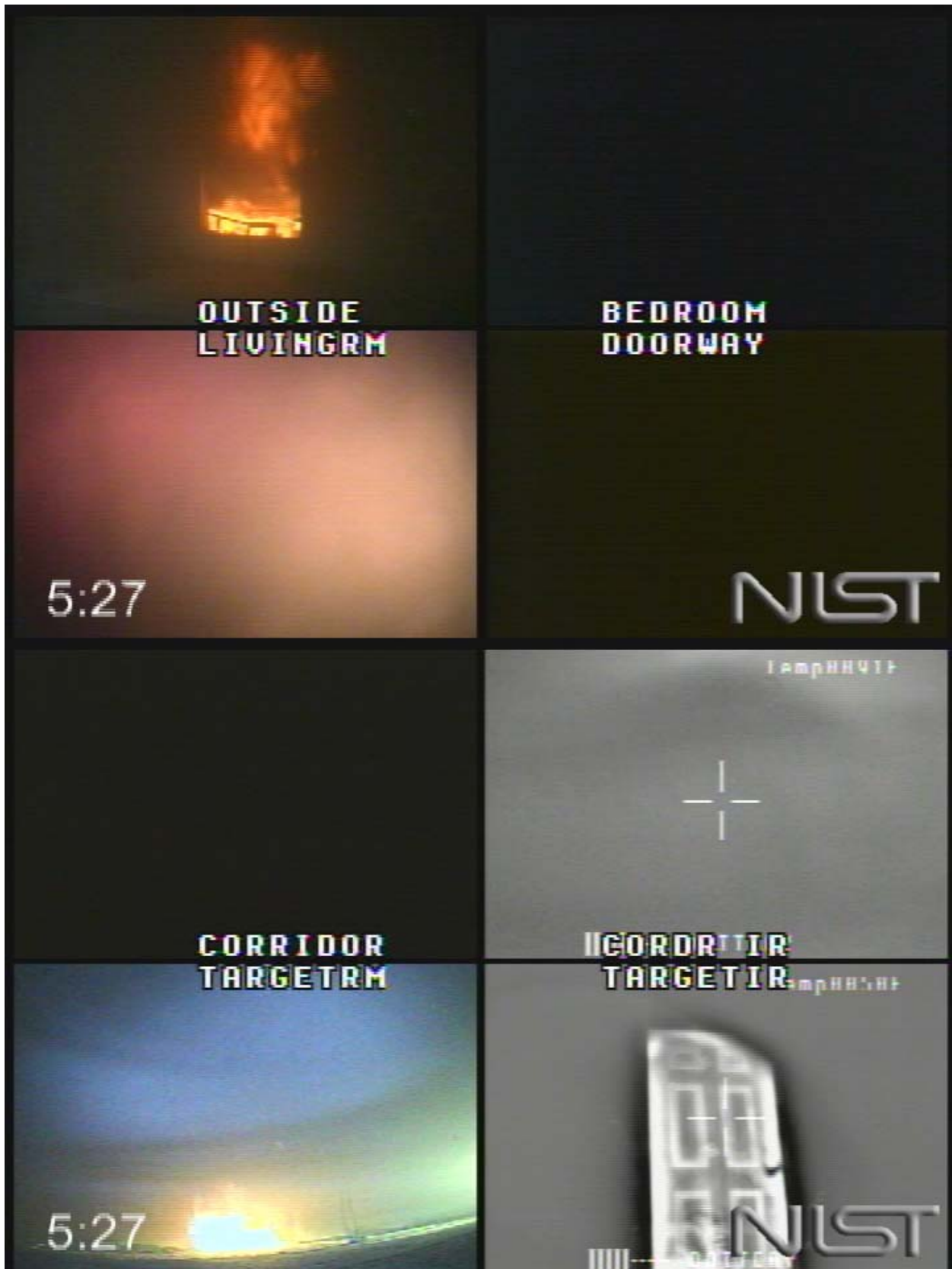
Figure 5.5.1-8. Experiment 5, WCD deployed; 327 s after ignition.
