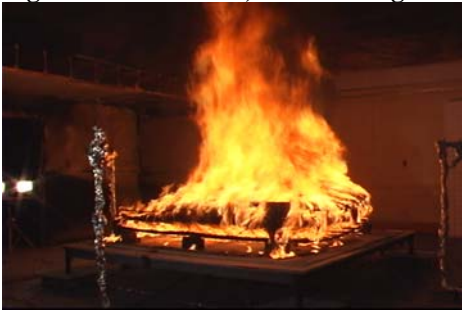
Figure 3.3.2-5. Bed 2, at peak heat release rate, 380 s after ignition
