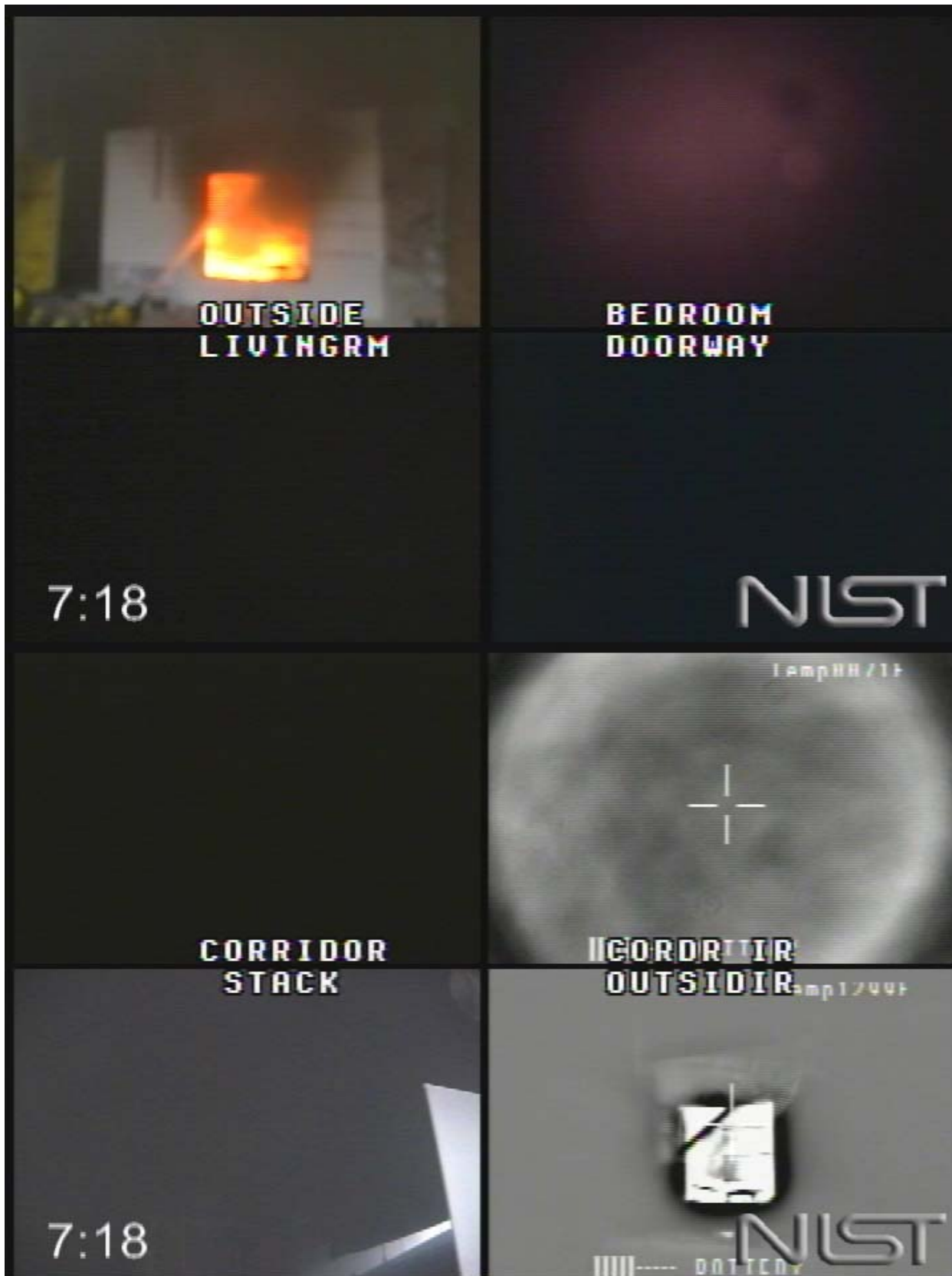
Figure 5.7.1-10. Experiment 7, indirect suppression started, 438 s after ignition.
