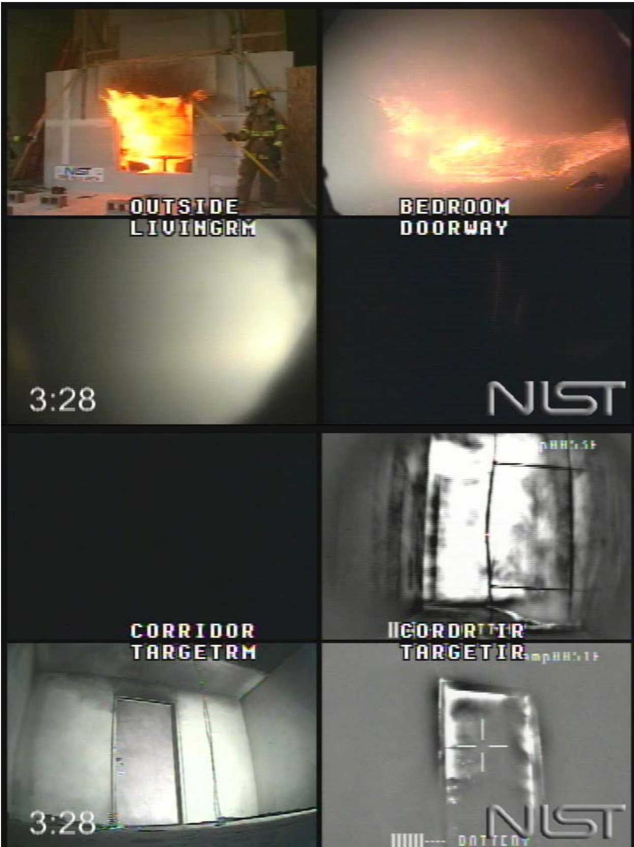
Figure 5.3.1-5. Experiment 3, window fully vented, 208 s after ignition.
