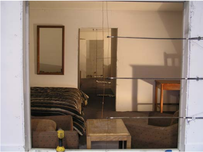
Figure 4.1.3-3. Bi-directional probe array in west window.
