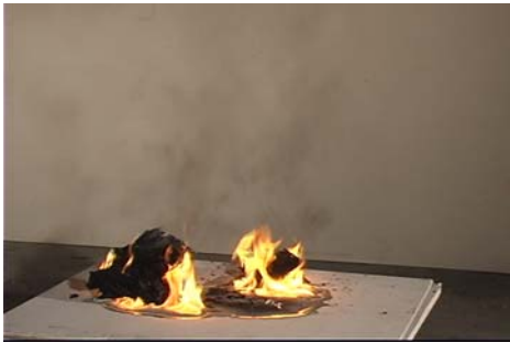
Figure 3.2-16. Trash container 2, 600 s after ignition
