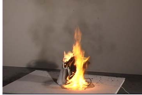
Figure 3.2-4. Trash container 1, 300 s after ignition
