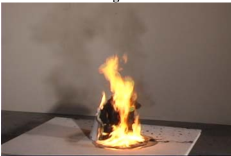
Figure 3.2-5. Trash container 1, 400 s after ignition
