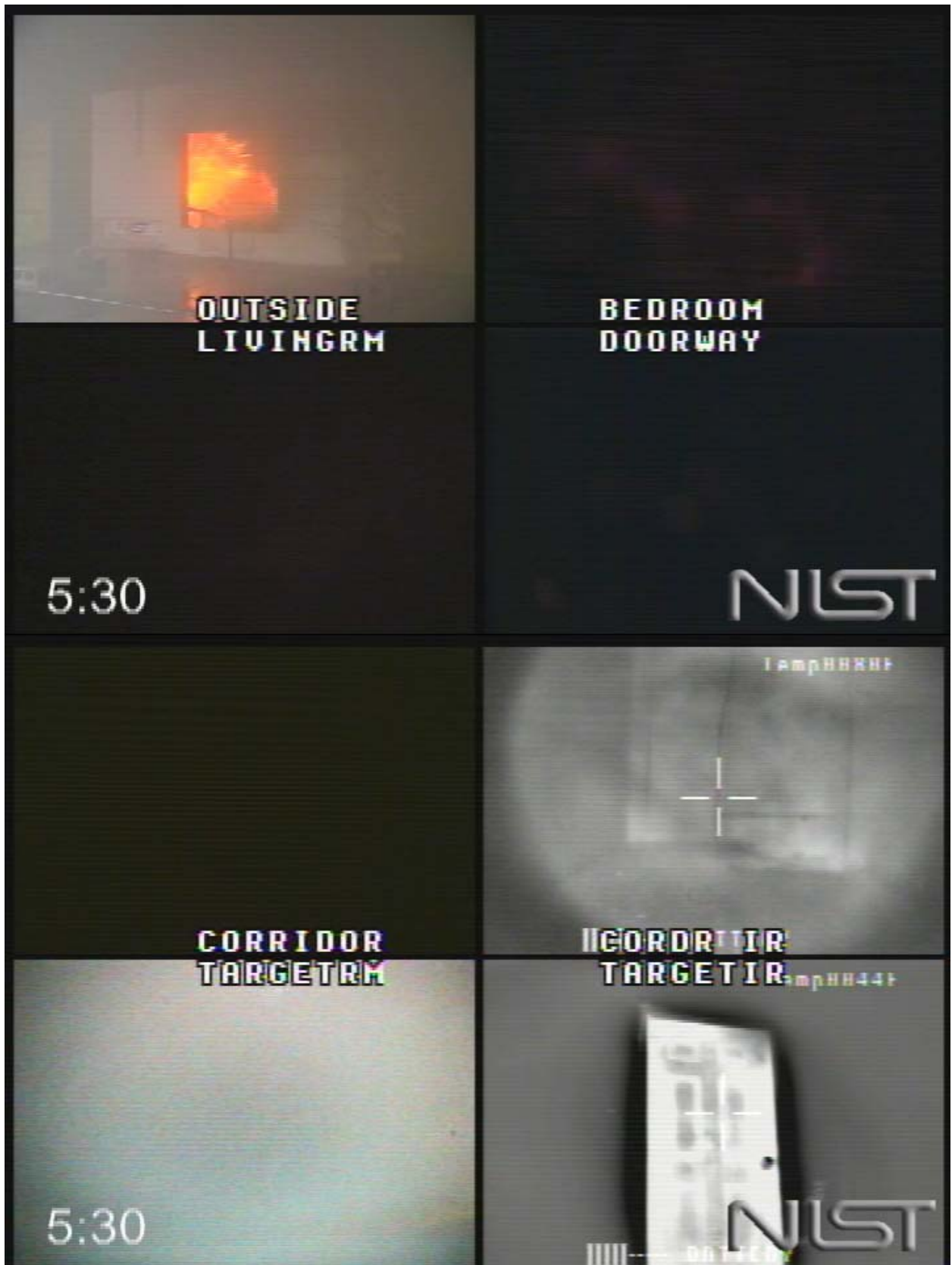
Figure 5.6.1-11. Experiment 6, fog stream across window off, 330 s after ignition.
