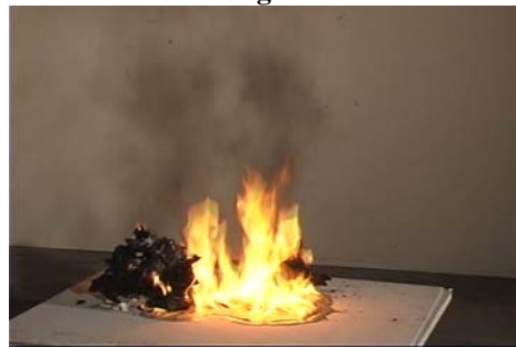
Figure 3.2-6. Trash container 1, at peak heat release rate, 406 s after ignition
