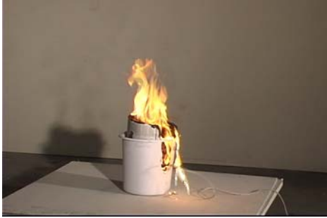
Figure 3.2-10. Trash container 2, 100 s after ignition
