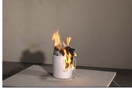
Figure 3.2-2. Trash container 1, 100 s after ignition
