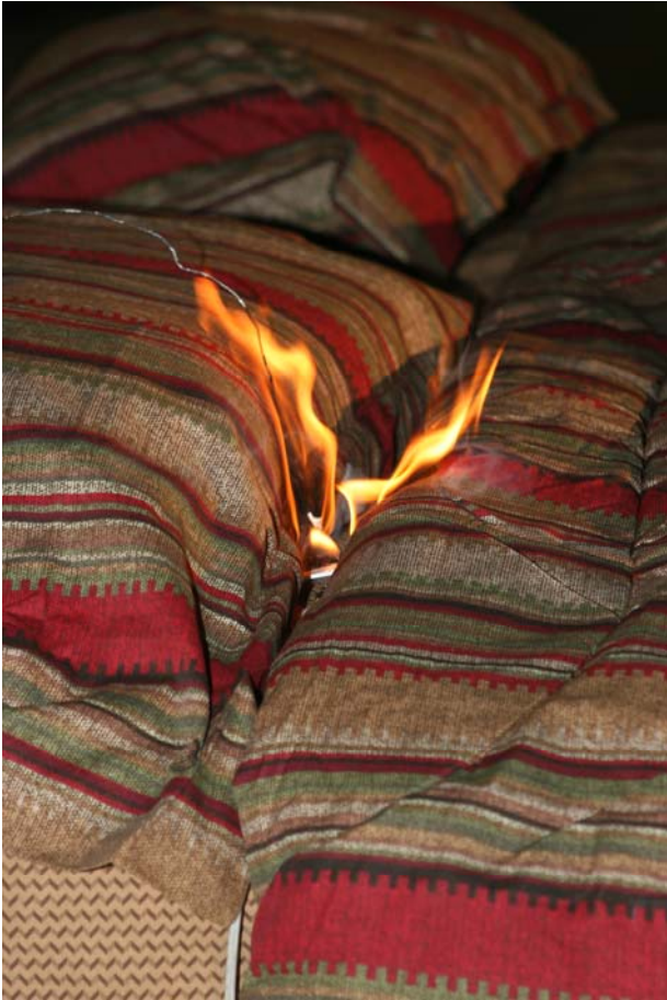
Figure 3.3-3. Electric match ignition of bed fuel package.
