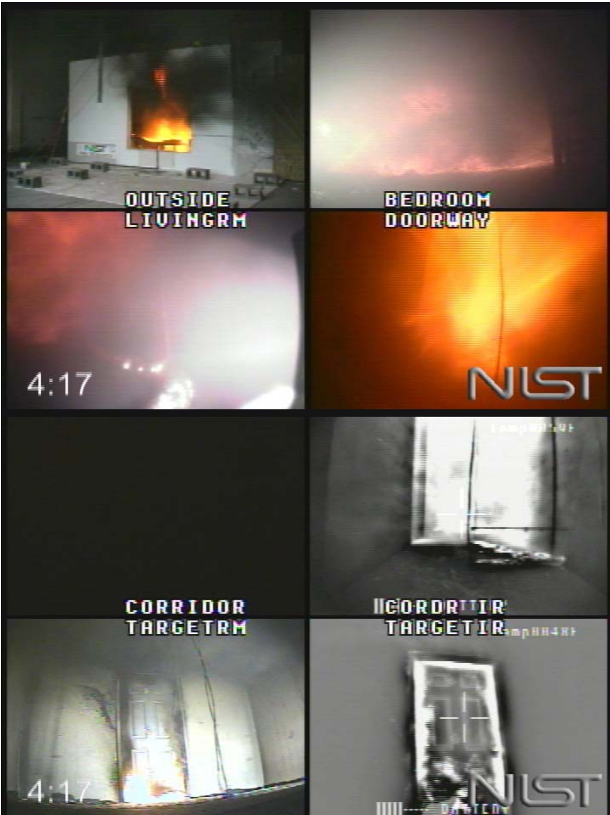
Figure 5.5.1-6. Experiment 5, corridor flames, 257 s after ignition.
