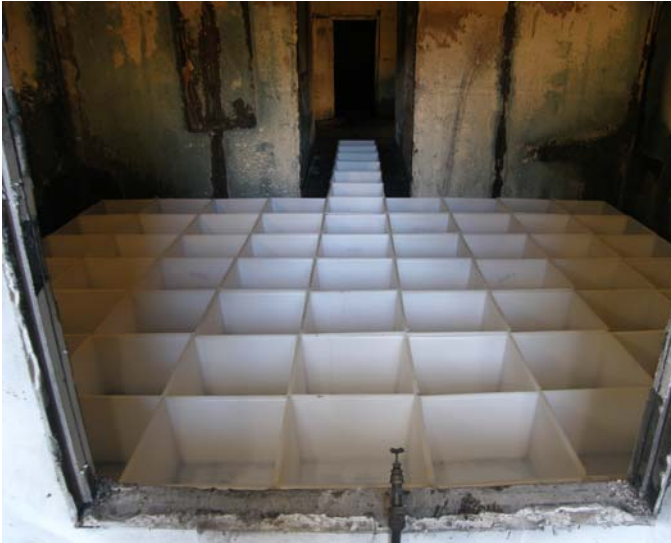
Figure 4.3.3-1. Water spray distribution experiment arrangement.
