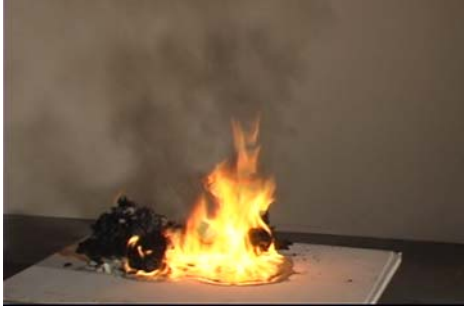
Figure 3.2-14. Trash container 2, 400 s after ignition
