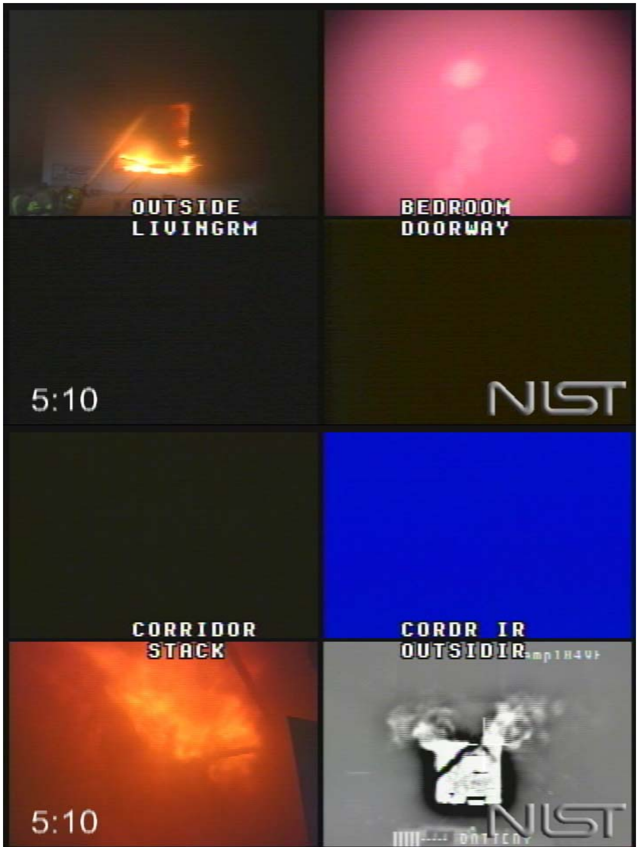
Figure 5.8.1-9. Experiment 8, indirect suppression started, 310 s after ignition.
