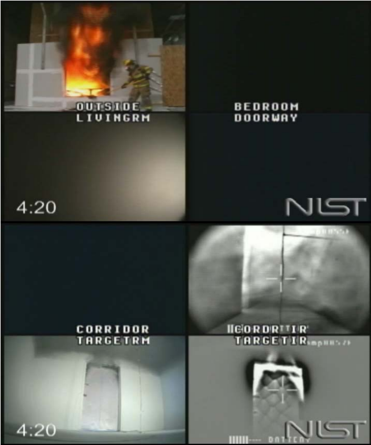
Figure 5.1.1-6. Experiment 1, window fully vented, 260 s after ignition.
