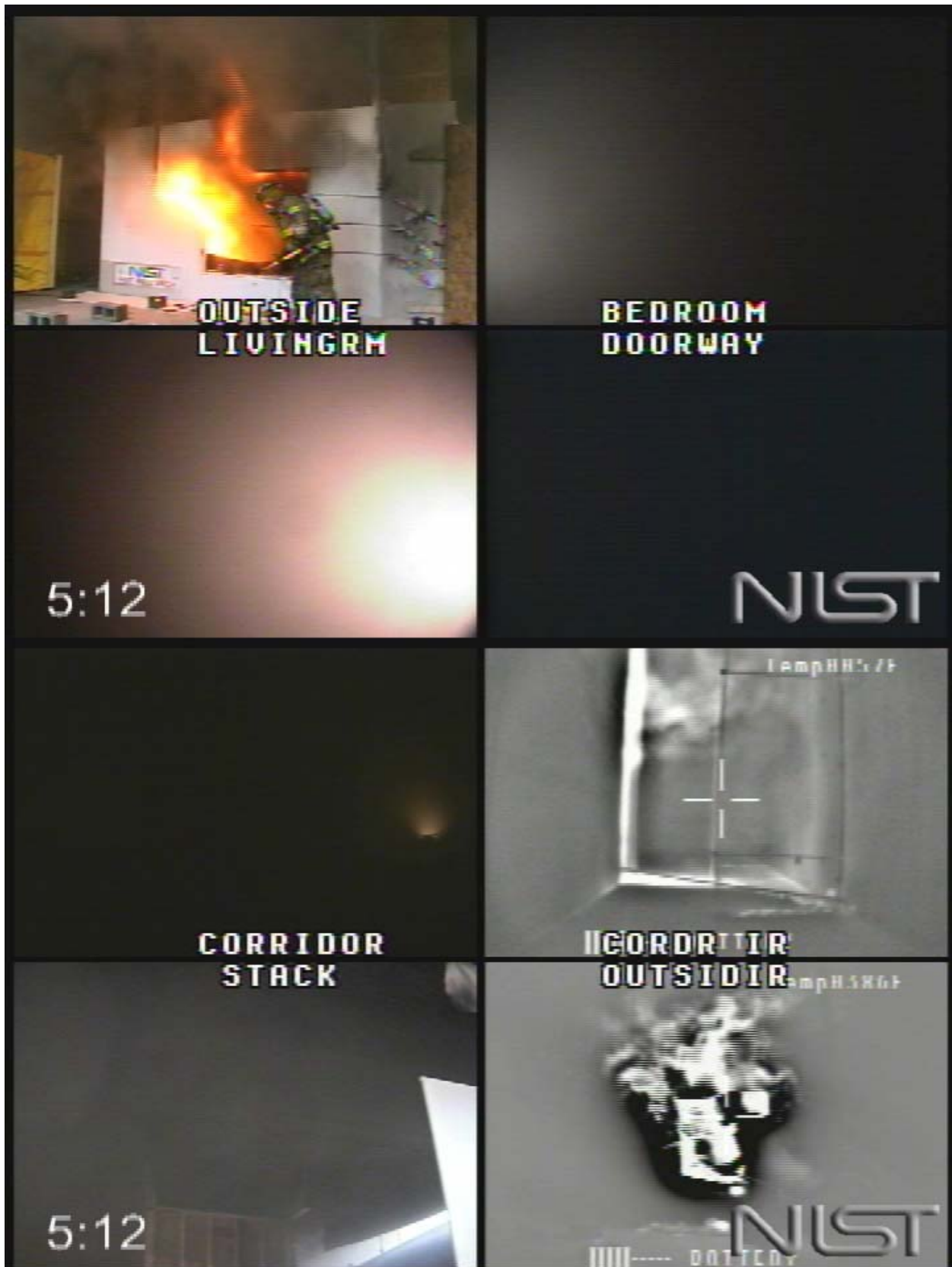
Figure 5.7.1-7. Experiment 7, window fully vented, 312 s after ignition.
