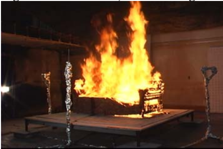
Figure 3.5-15. Sofa 2, at peak heat release rate, 389 s after ignition
