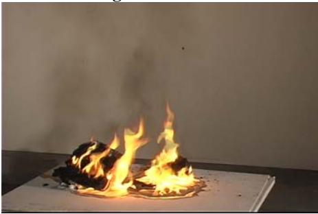
Figure 3.2-15. Trash container 2, 500 s after ignition
