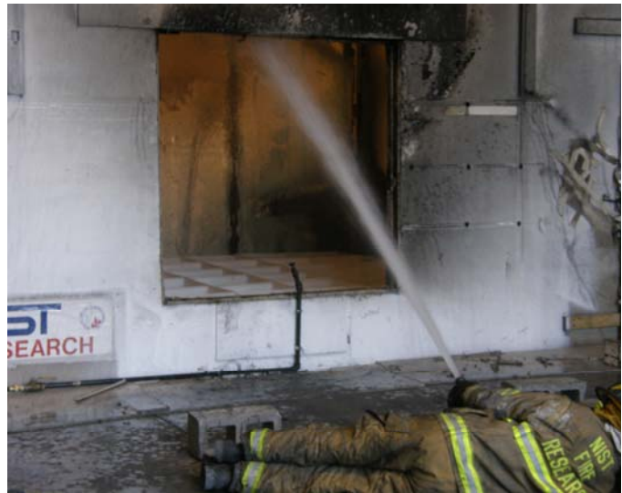
Figure 4.3.3-4. Solid stream discharged into window opening.
