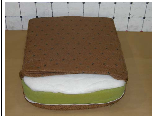
Figure 3.4-3. Seat cushion, showing layers of upholstery fabric, polyester batting and polyurethane foam.
