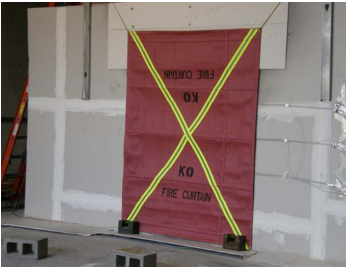
Figure 4.3.2-1. Small WCD deployed over window opening.
