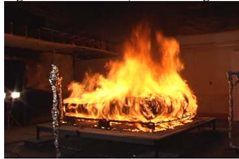
Figure 3.3.1-6. Bed 1, at peak heat release rate, 484 s after ignition
