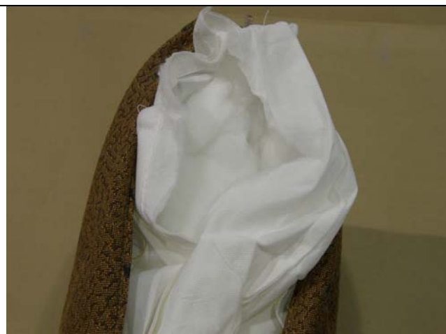
Figure 3.4-4. Back cushion, showing the upholstery fabric, inner liner, and polyurethane foam.
