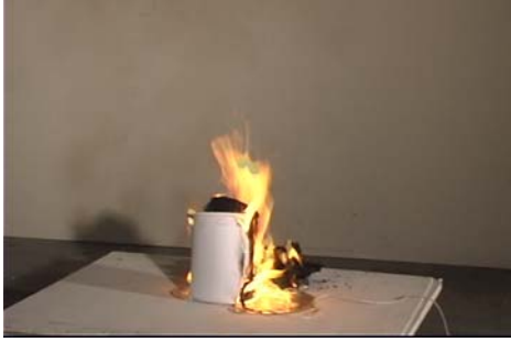
Figure 3.2-12. Trash container 2, 300 s after ignition
