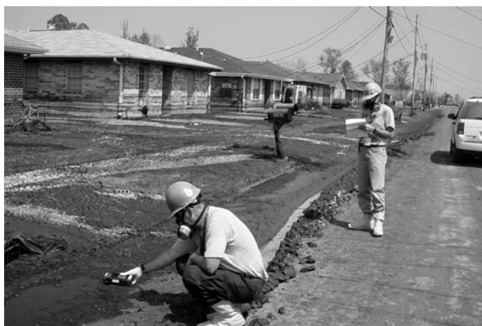
Figure 9: OSHA Field Staff Sampling the Air, Water, and Soil on the Gulf Coast by Pinning a Small Personal Monitor to a Worker, Taking Water Samples, and Taking Soil Samples
