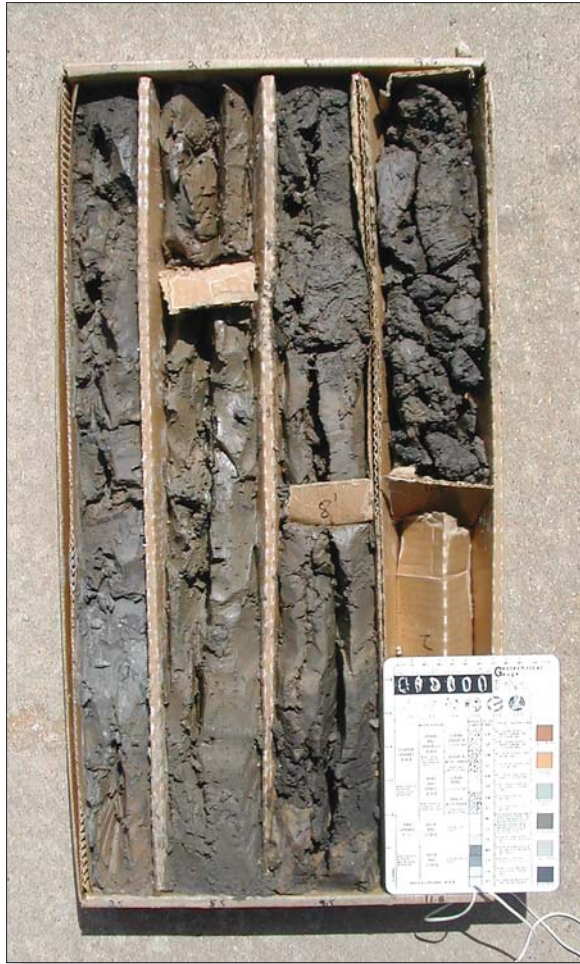
Figure 6. Example of lithologic core collected from hoverprobe boring site DCHP01 on a tidal flat in the Anacostia River north of Benning Road, Washington, D.C., July 2, 2002. (Photo by Daniel Phelan, USGS)
