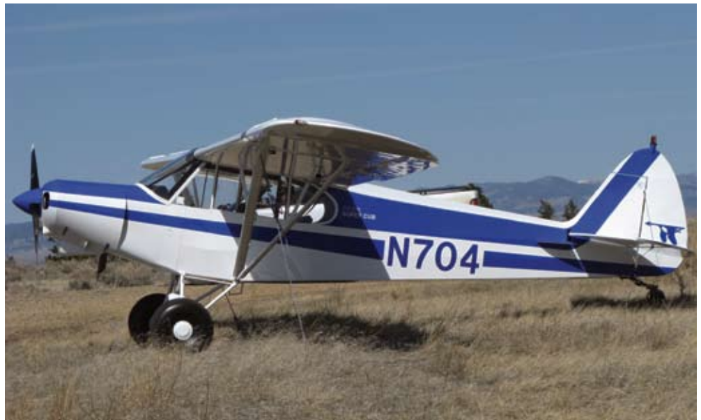
This rebuilt Piper Supercub is the preferred equipment for refuge pilots because of its slow flight capability, enhanced visibility, crashworthiness and simple design. (USFWS)
