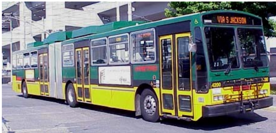
Figure 4. Refurbished Breda Dual-Mode Bus to Electric-Only Trolley-Bus Operation
