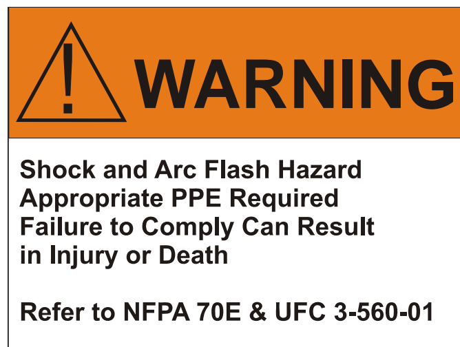
Figure 4-1. Arc Flash Warning Label
