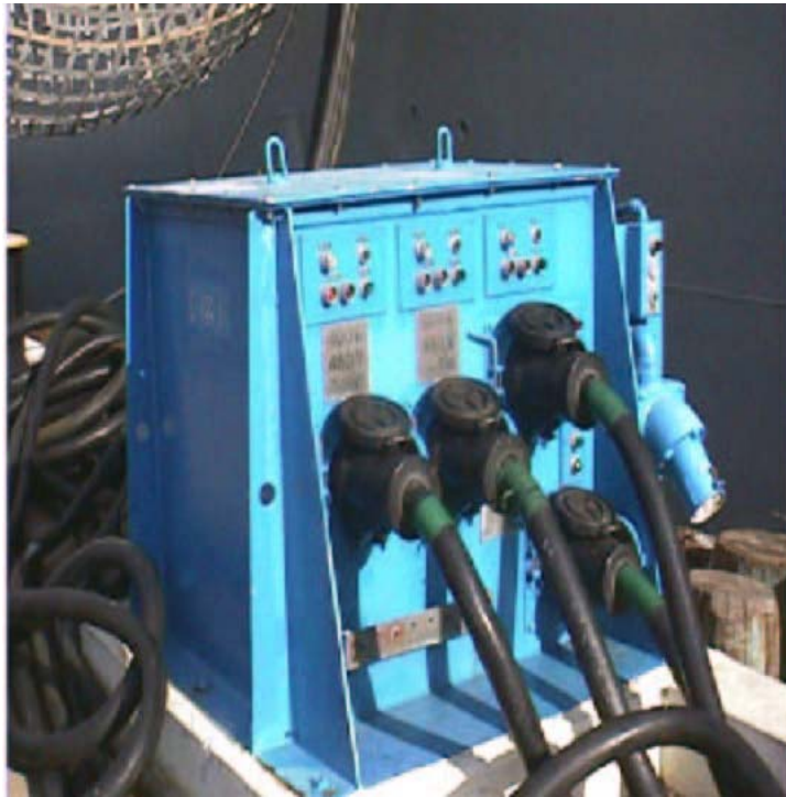
Figure 13-11. 480 Volt Shore-Cable to Ship-Cable with Single-Pole Connection
