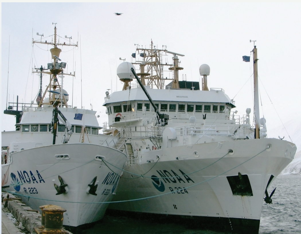
▲ NOAA ships Miller Freeman (left) and Oscar Dyson (right) in Dutch Harbor, Alaska. Although the ships are of similar length, the Dyson has approximately 30% more displacement and approximately 40% more horsepower.
