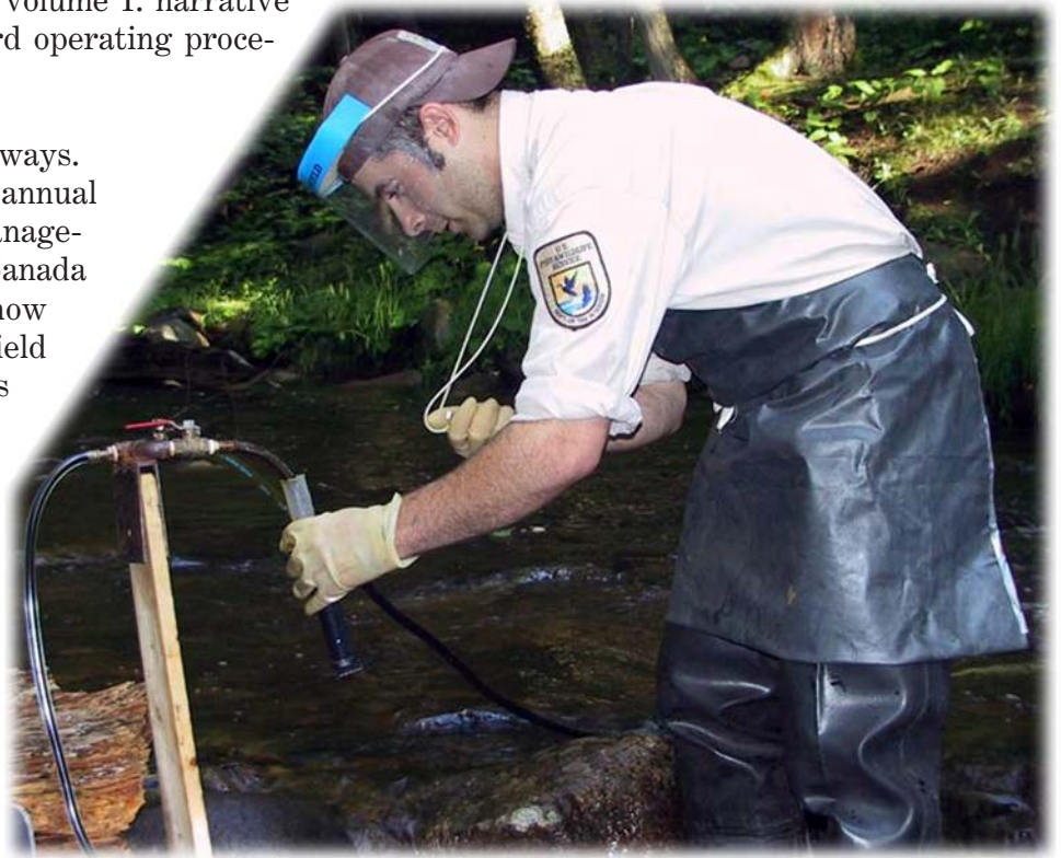
-GLFC Technician Wayne Stanislawski of the Marquette Biological Station measures the application rate of lampricide during a typical stream treatment. All aspects of lampricide application as well as training and safety procedures are detailed in the manual of standard operating procedures.
