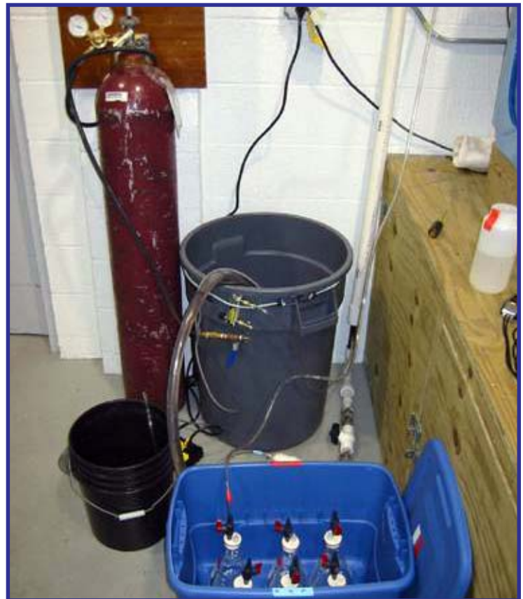
Small-Scale VOS System with Light-tight Container and Six Identical One Liter Flasks
