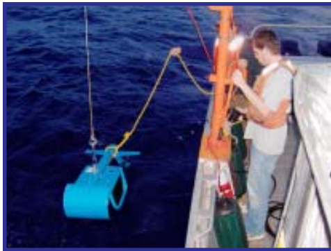
-USFWS Ashland Fishery Resources Office prepares to collect acoustic data to measure cisco densities in western Lake Superior.
