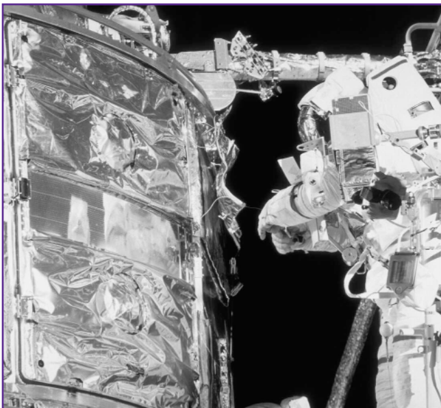
Astronaut Repairing Insulation During Servicing Mission 2
