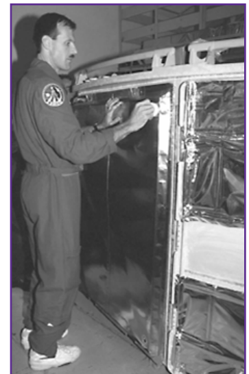
Astronaut Steve Smith installing a sheet of NOBL on the Hubble Mockup
