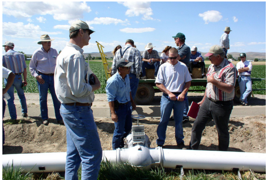
Local producers discuss the benefits of improved irrigation systems, such as gated pipe and surge to conserve water.
