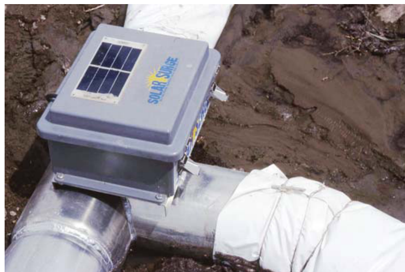
Solar surge valve used to regulate distribution of water for increased efficiency.
