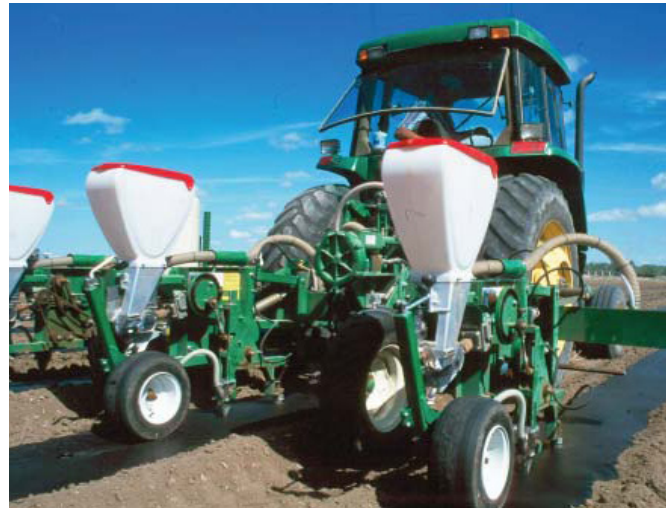
Burning holes into plastic and planting seed melons in a drip irrigation system to conserve water.
