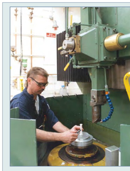
An HE machinist gauges a tensile specimen to check for tolerance.
