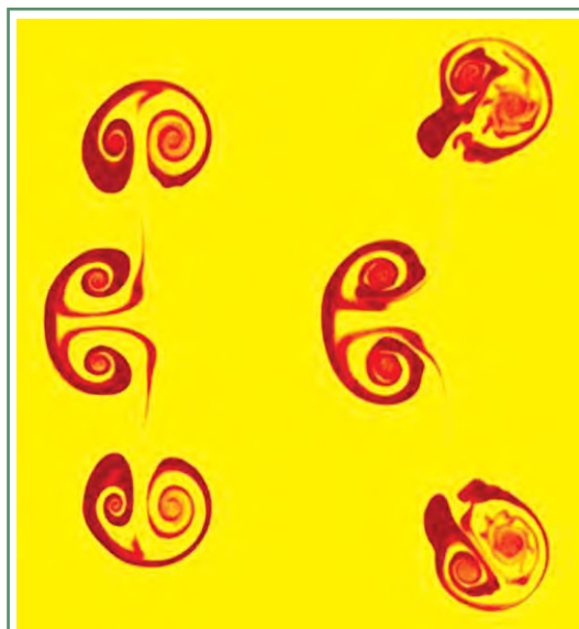
Figure 1. When a planar shock wave impacts three gas cylinders, it creates the three vortex pairs, seen in cross section, by illumination with a thin sheet of laser light. These successive snapshots of the vortex pairs at an earlier time (left) and later time (right) show how the flows become highly distorted en route to turbulence.
