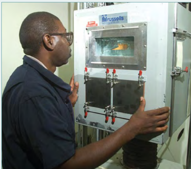
A mechanical testing technician closes an environmental chamber door and sets temperature before initiating a quasi-static tension or compression test.
