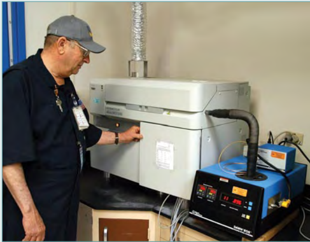
A chemical technician measures binder molecular weight using size exclusion chromatography/gel permeation chromatography.
