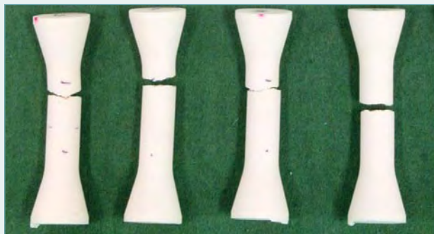
High-explosive "dog bone" specimens after quasi-static tension testing.
