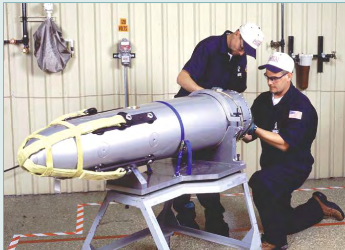
Surveillance identifies and examines signs of aging in components removed from weapons during disassembly at the Pantex Plant.
