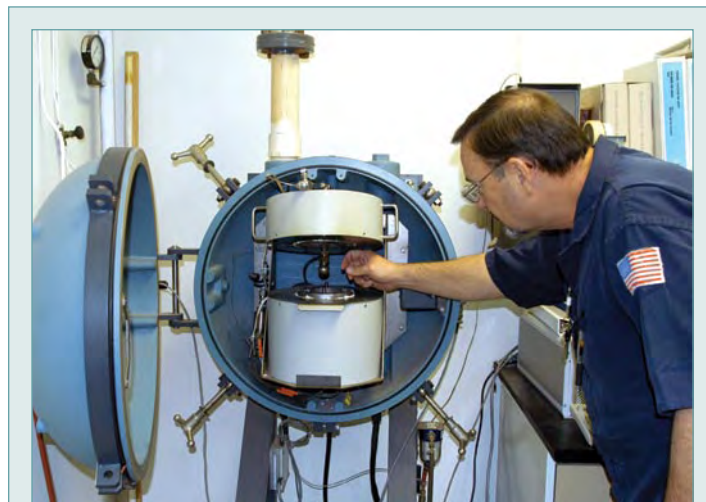
A chemical technician loads the accelerated rate calorimetry chamber.
