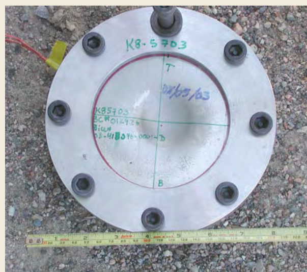
Digital images from quenched, X-0557-1.6 Target K8-5703 showing (top) target intact and attached to backing plate and ballistic pendulum and (lower) evidence of cover plate indentation by projectile impact.
