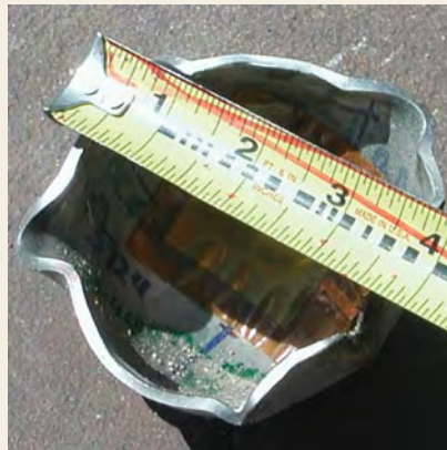
Digital images from post-test X-0557-2.0 Target K8-5724 after HEVR showing (top to bottom) target holder, retaining ring, and cover plate damage. In some tests, the target damage was comparable to PBX 9501 baseline tests; in others, physical damage and energy release exceeded baseline results.
