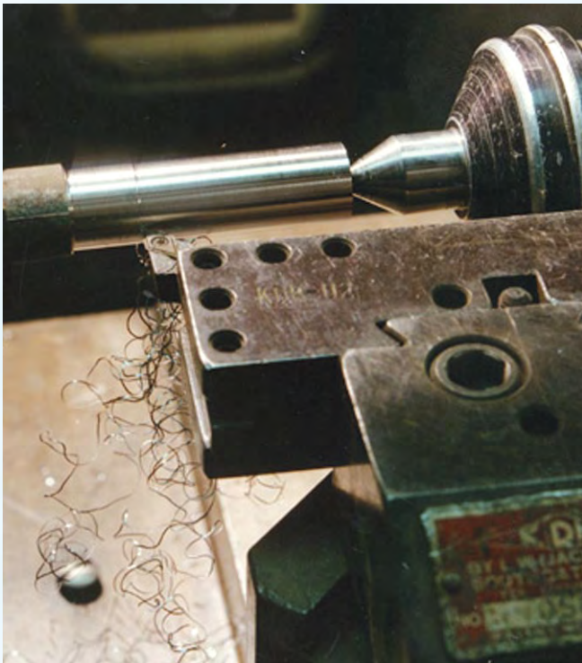
Plutonium part being created with the dry-machining process developed at Los Alamos.
