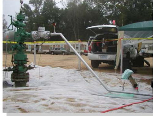
Perfluorocarbon Tracers are Added to CO 2 as it is Injected at the Frio Test Site Near Houston, TX
