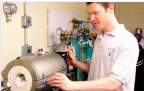
Danvers Johnston, an IGERT program fellow in the laboratory at the Nano/Bio Interface Center at the University of Pennsylvania, creates nanotubes by reacting methane and hydrogen gas with nanometer-diameter iron catalyst particles. Credit: The Nano/Bio Interface Center at the University of Pennsylvania.
