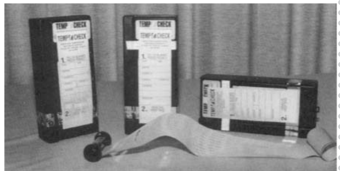
Figure 14 Analog disposable recording temperature monitors which use a battery powered motor to pull a strip chart. The chart is obtained by breaking open the recorder box.
