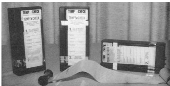
Figure 29 The box must be broken open and the strip chart removed to determine the temperatures reached during shipping. (See accompanying text.)
