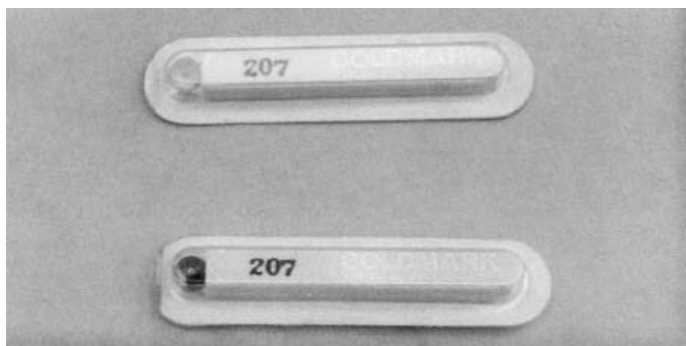
Figure 28 The top indicator is clear, the bottom indicator means the vaccines have been too cold at some point during shipping. (See accompanying text for more information.)
