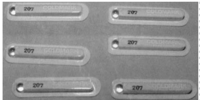
Figure 13 A color-change monitor releases an irreversible red dye if the temperature inside the package reaches the freezing point of water.
