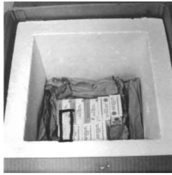
Figure 24 Place a heat monitor (outlined in black) close to the vaccines, but away from the cold packs.
