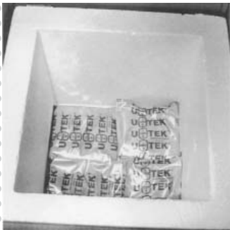
Figure 22 Put 4 cold packs on the bottom of a large box for warm weather shipping of the vaccine.
