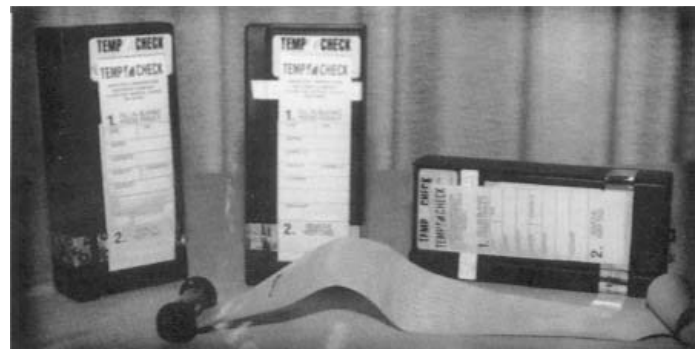
Figure 32 Analog disposable recording temperature monitors. The monitor must be broken open to get the chart strip inside.
