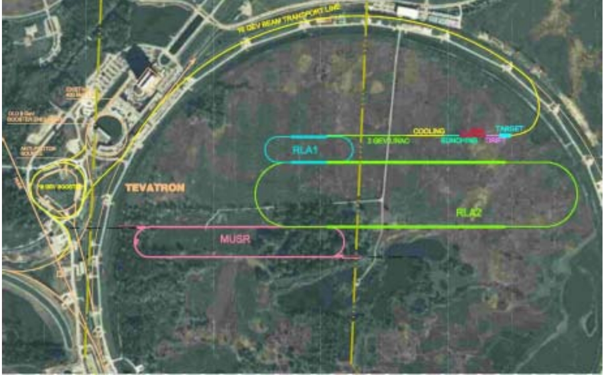
FIG. 23: Schematic of a 50-GeV Neutrino Factory at Fermilab.
