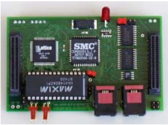
▲ Generic ARCNET board used for intelligent general purpose control in the high magnetic field environment of PHENIX.
