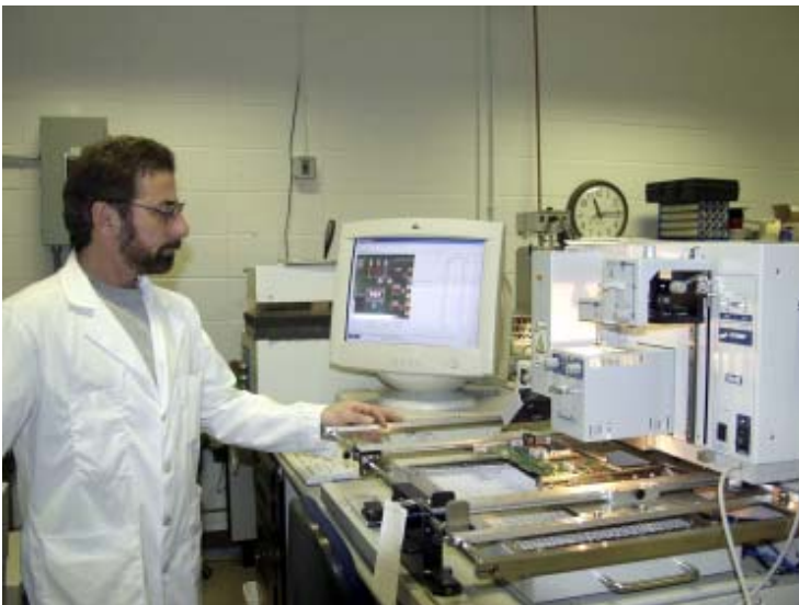
▲ John is demonstrating the x-ray circuit board inspection station and the BGA re-work station.
