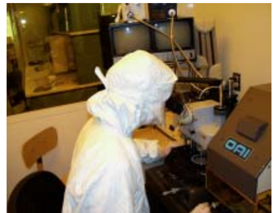
▼ Double-sided mask aligner station in the Class 100 cleanroom facility.
