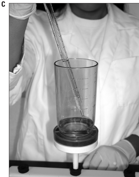
Figure 7.1-3. Steps in membrane-filtration procedure.
