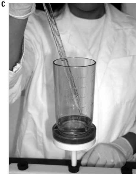
Figure 7.1-3. Steps in membrane-filtration procedure.
