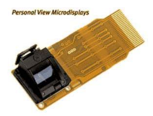
An FLC display chip, sitting atop a silicon wafer, is smaller, faster, uses less power, and can be magnified to extrememly large sizes without image degradation.
