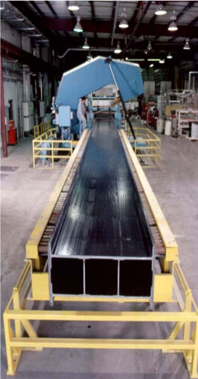
The double-web I design improved performance, increased the shear load distribution capability of the beam, and improved the stiffness, making the beam resistant to bending; and therefore very useful in building bridges.
