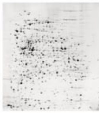
Figure 1. 2D gel following electrophoresis of a cell lysate. Figure courtesy of Dr. Timothy Veenstra, Laboratory of Proteomics and Analytical Technologies
