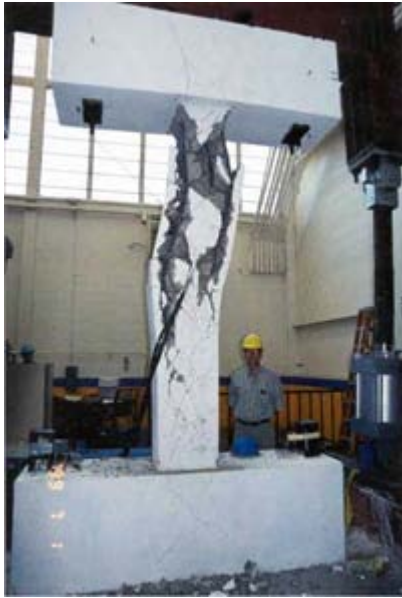
Laboratory testing of an older concrete column design. Photo copyright 2002 by Pacific Earthquake Engineering Research Center.
