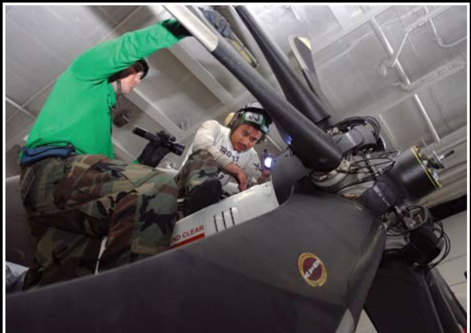
AE1 Josh Deitrick and AD2 Mikhos Maneru, both assigned to the "Wall-bangers" of VAW-117, perform propeller maintenance on an E-2C Hawkeye aboard the aircraft carrier USS Nimitz (CVN-68). Navy photo by MC3 J. D. Levite
