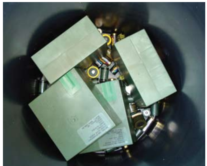
The wrong way: Lithium batteries stored alongside other types of batteries.
