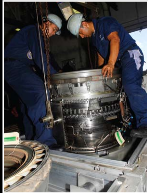
ADAN Joan Medina, left, and AD3 Elman Pena perform a level III preservation on the NRFI F-414 fan module of a turbo-fan engine from an FA-18F Super Hornet aboard the aircraft carrier USS John C. Stennis (CVN-74). Navy photo by MC3 Kenneth Abbate
