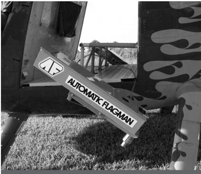
Helicopter with dispensers for aerial delivery of dead mouse flag-baits to brown treesnakes. (Photo by: Ken Tope, USDA)
