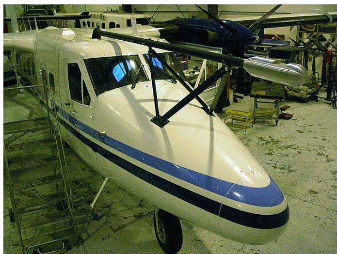
New boom and BAT probe installed on NOAA Twin Otter.
