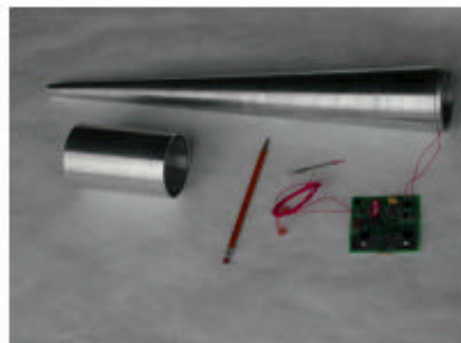
Figure 1. Refractive turbulence - high speed temperature probe.
