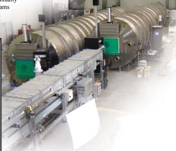
Left: schematic of the Powder Diffractometer at HFIR, which is scheduled for initial commissioning by fall 2007. Center: detector tanks for the new SANS instruments. On the left is the general-purpose, high-resolution instrument; on the right is the SANS instrument constructed specifically for biological research. Top right: schematic of the guide tubes leading into the SANS instrument detector tanks.
